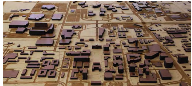
Figure 13. Fabricated physical model of Texas A&M University campus from the BIM which is inherited from GIS data.
