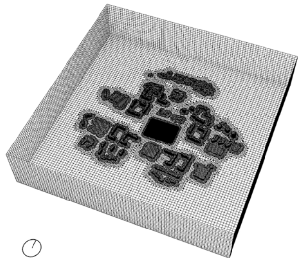
Figure 4. The domain used for CFD simulations. In the center the area of interest characterized by a highly refined mesh surrounded by context buildings for which a larger refinement mesh is used.
