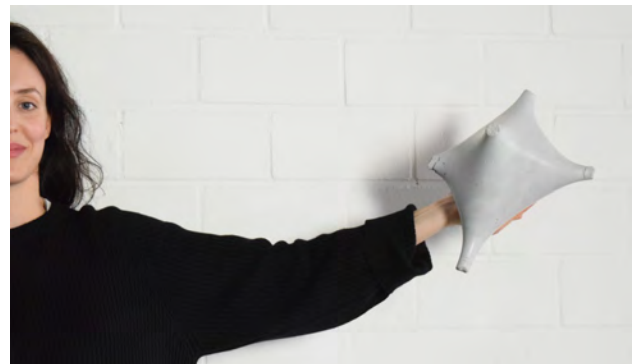
Figure 1. A lightweight hollow concrete (UHPC) object rotoformed in a prestressed latex membrane.
