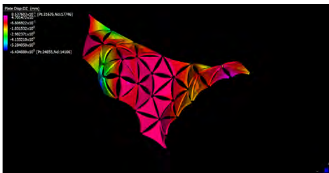
Figure 7. Vertical displacement of structure under self-weight.
