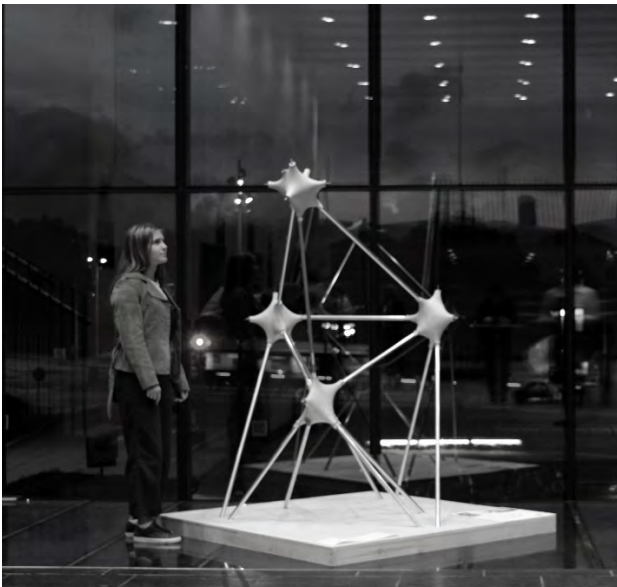
Figure 9. The large scale demonstrator of space truss system at AAG Conference 2018 with hollow body concrete nodal component
