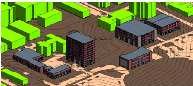
Figure 11. The non-geometric information which the BIM objects inherit from GIS can be used for automated façade design.
