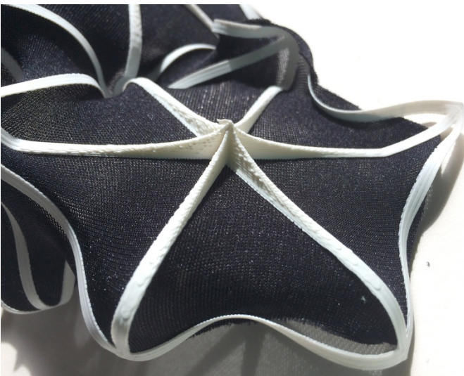
Fig.15. 3D printed sample with a gradual height change
