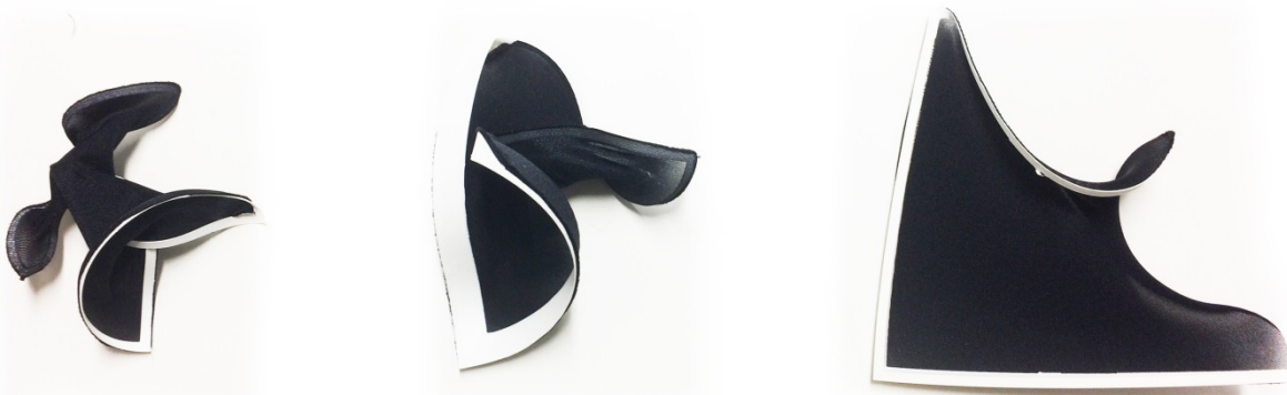
Fig.06. Three modules of 18,5 x 18,5 cm each with various 3D printed edge thickness (left: the same thickness of all the four edges: W: 5mm, H:0,6mm, middle: two edges W: 5mm, H:0,6mm and two wider ones: W: 15mm, H:0,6mm, right: 2 edges W: 5mm, H:0,6mm and two higher ones: W: 5mm, H:8 mm)
