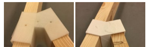
Fig.9: Sequence of 3d print joints supporting the spatial structure.
