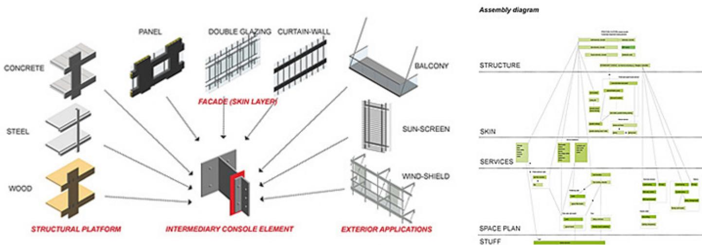
Fig. 6: Illustration of intermediary element.
