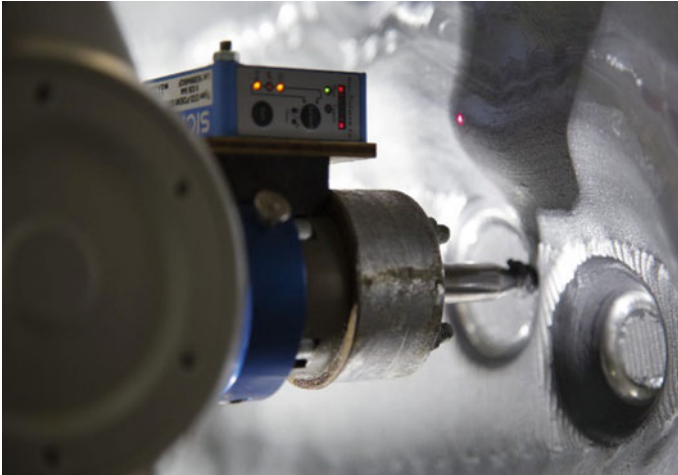
Fig. 2. Single point distance sensor mounted to the robot arm
