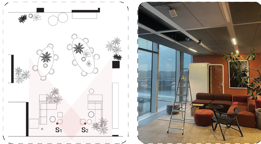
Figure 6: The positioning of the two Kinect cameras, along with a picture of the setup.
