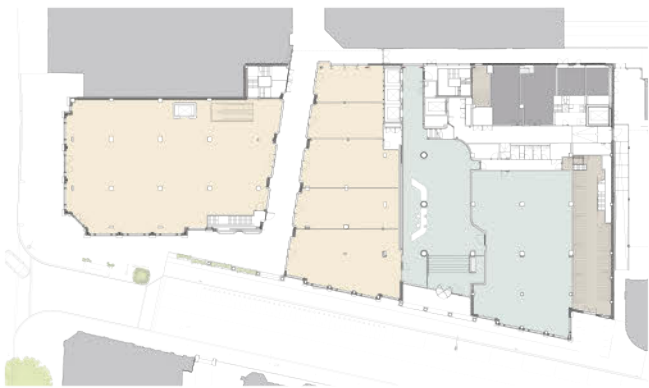
Ground floor with office entrance at 1 Wright's Lane and retail fronting Kensington High Street and the new arcade linking to the Underground station.
