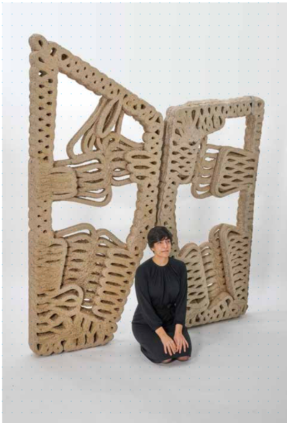
The biopolymer screens printed at COBOD are 2.3m high and weigh 35kg each.
