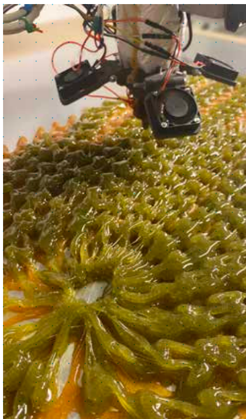
Experiment with bone glue printing using different colours at CITA
