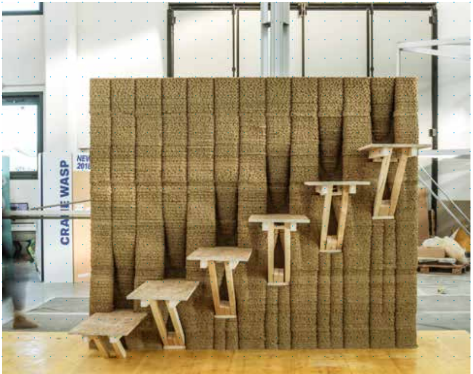
Full-scale prototype of novel construction system using 3D-printed earth and timber (IAAC 3DPA with WASP)
