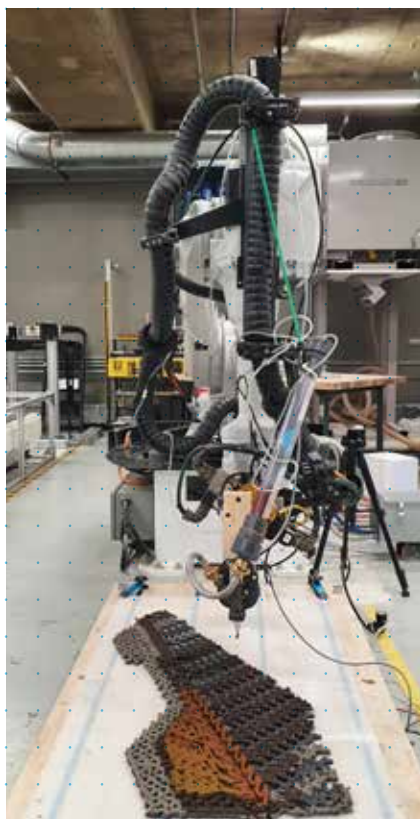
Grading by fibre content of printed cellulose in CITA workshop at University of Pennsylvania
