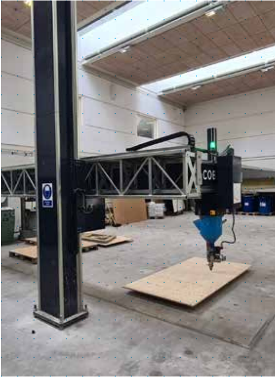
The cellulose and Xanthan-based slurry can be processed by large-scale concrete printers such as the COBOD printer which has a printing range of up to 20m × 24m.
