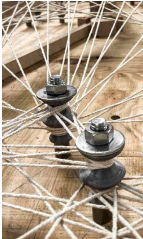
Test of the node detail carrying a lightweight building element made of timber and wound natural fibre
