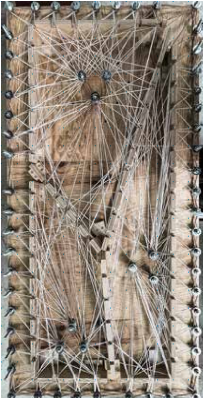
Scale model used to develop the fibre matrix of the ITKE-FibR Living Prototype
