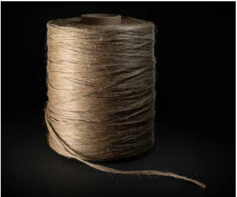
Robotic fibre-winding fabrication works with flax fibres prepared as yarns.
