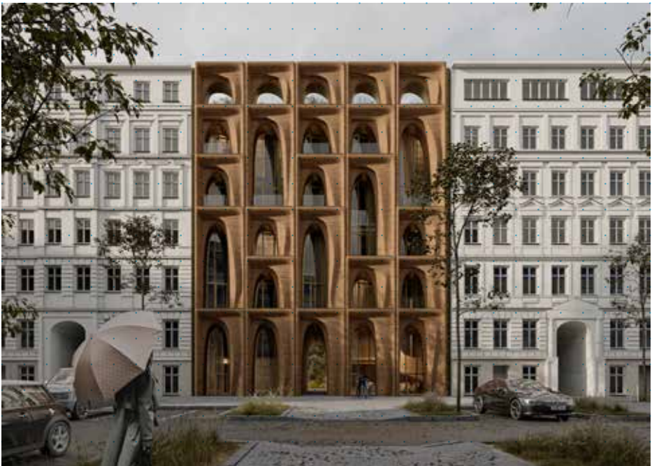
Speculative design for an earth-printed façade in Berlin (IAAC 3DPA)
