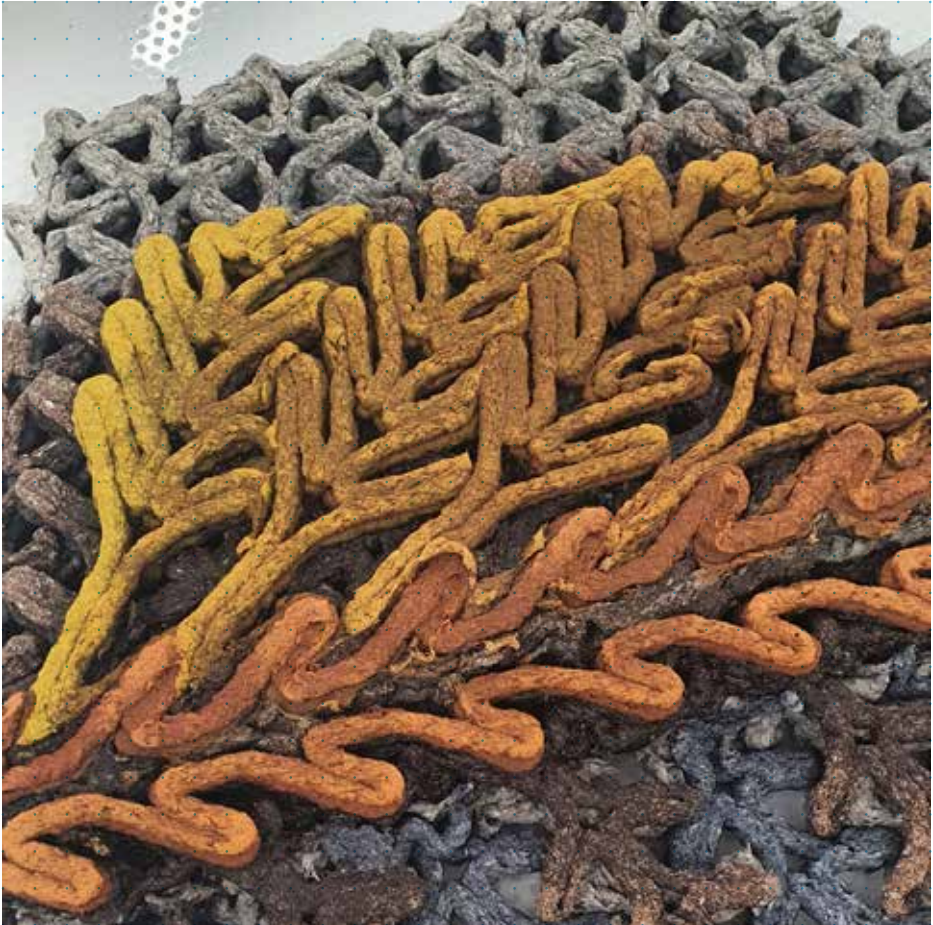
Gradient-print made of cellulose and varying natural fibres, produced in CITA workshop at University of Pennsylvania
