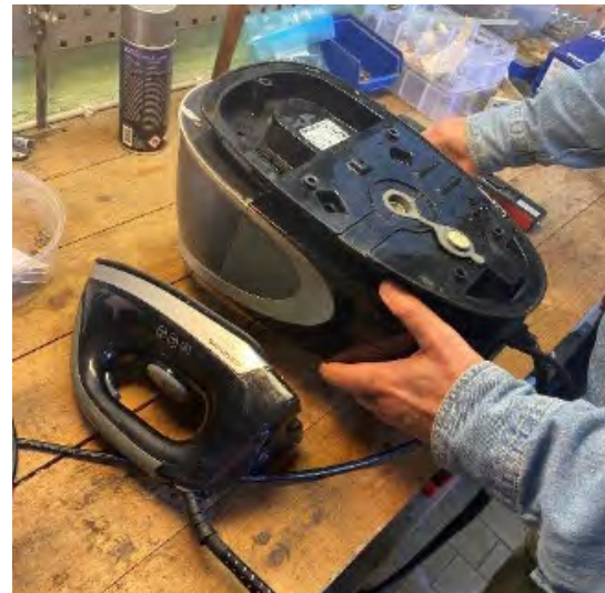
Figure 9. Declogging of a steamer
