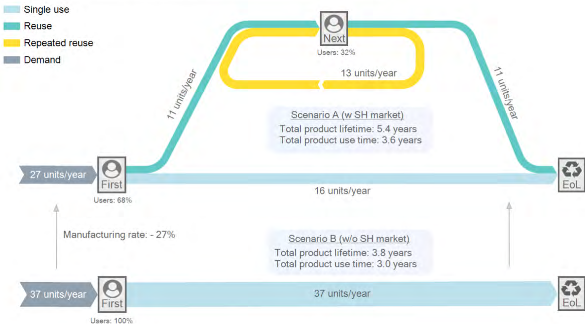
Figure 2. Sankey diagrams depicting the total demand for new smartphones and the flow between user types until products reach end-of-life in a benchmark scenario (A) based on surveyed consumer data and a scenario without a second-hand market (B) estimated from consumer data in a market with a population of P = 100 ; SH = secondhand.
