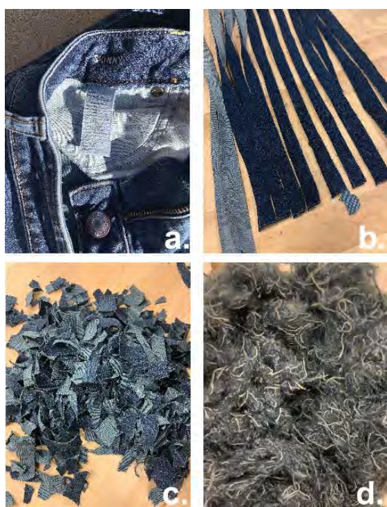
Figure 1. Textile transformation process: garment a) with fiber composition tag. b) cut into strips, c) cut into squares, d) shred into shoddy.
