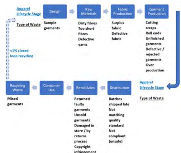
Figure 1. Simplified apparel supply chain model with examples of material waste at each stage. Adapted from Reverse Resources, 2017.
