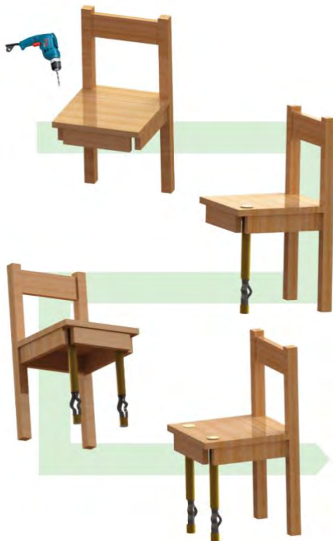
Figure 7. Repair process with replacement parts.
