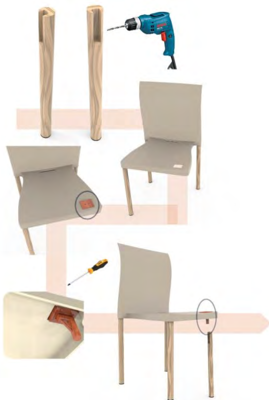
Figure 5. Repair process with connecting parts.
