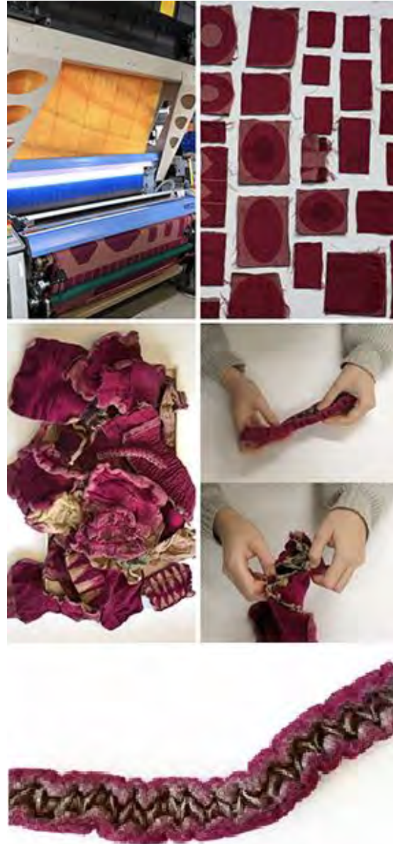
Figure 5. Top Left to Right: Weaving samples on industrial jacquard loom. Samples of the loom separated by cutting. Middle left to right: Samples after the felting process, displaying changes. Participants conducting the experiential characterization user study. Bottom: Detail of Ex. 1 sample.
