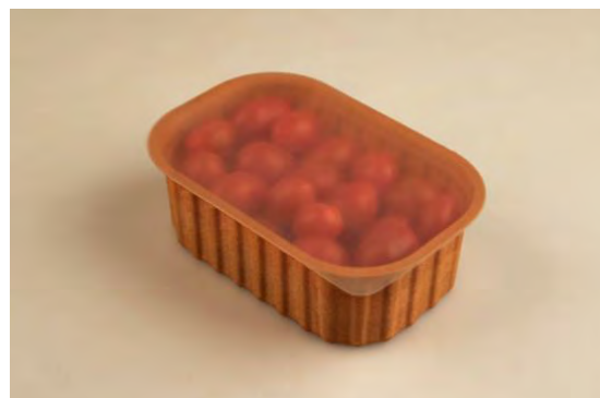
Figure 6. Case study #3: POMOPLA 2 3D printed packaging prototype.
