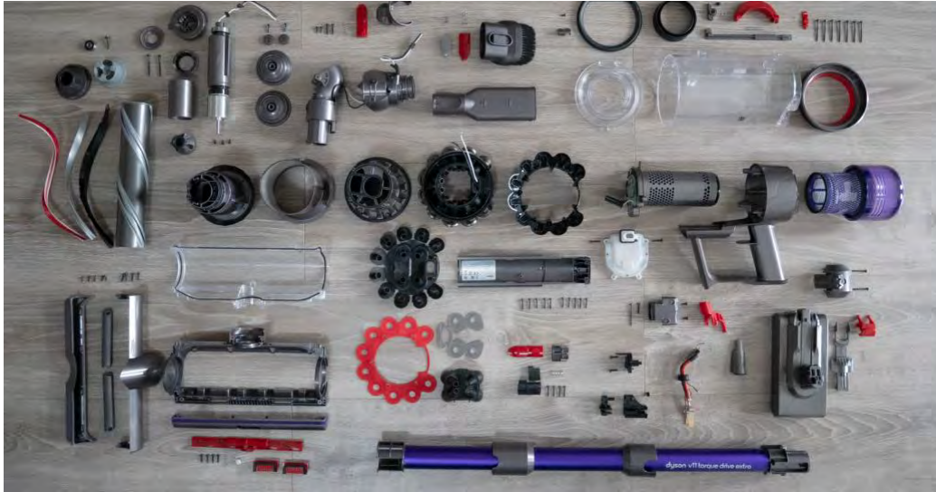
Figure 1. The disassembled Dyson V11.
