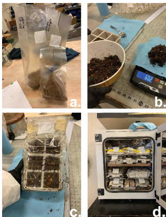
Figure 3. Mycelium composite manufacturing process: a) filtered bags before their sterilization; b) inoculation with grain spawn and weighing before filling silicone trays; c) filled silicone tray; d) incubation of trays in the Binder incubation chamber.
