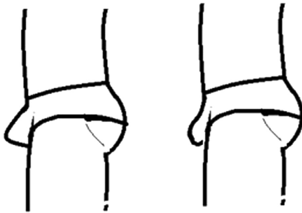
Figure 6: Two approaches to shaping the pouch profile. Left, active shaping achieved by locating the seam edge in a two-panel front. This design is associated with cotton or modal. Right, natural form-following 'passive' design using softer, more elastic fabric (thinner cottons, ribbed cotton, elastane).
