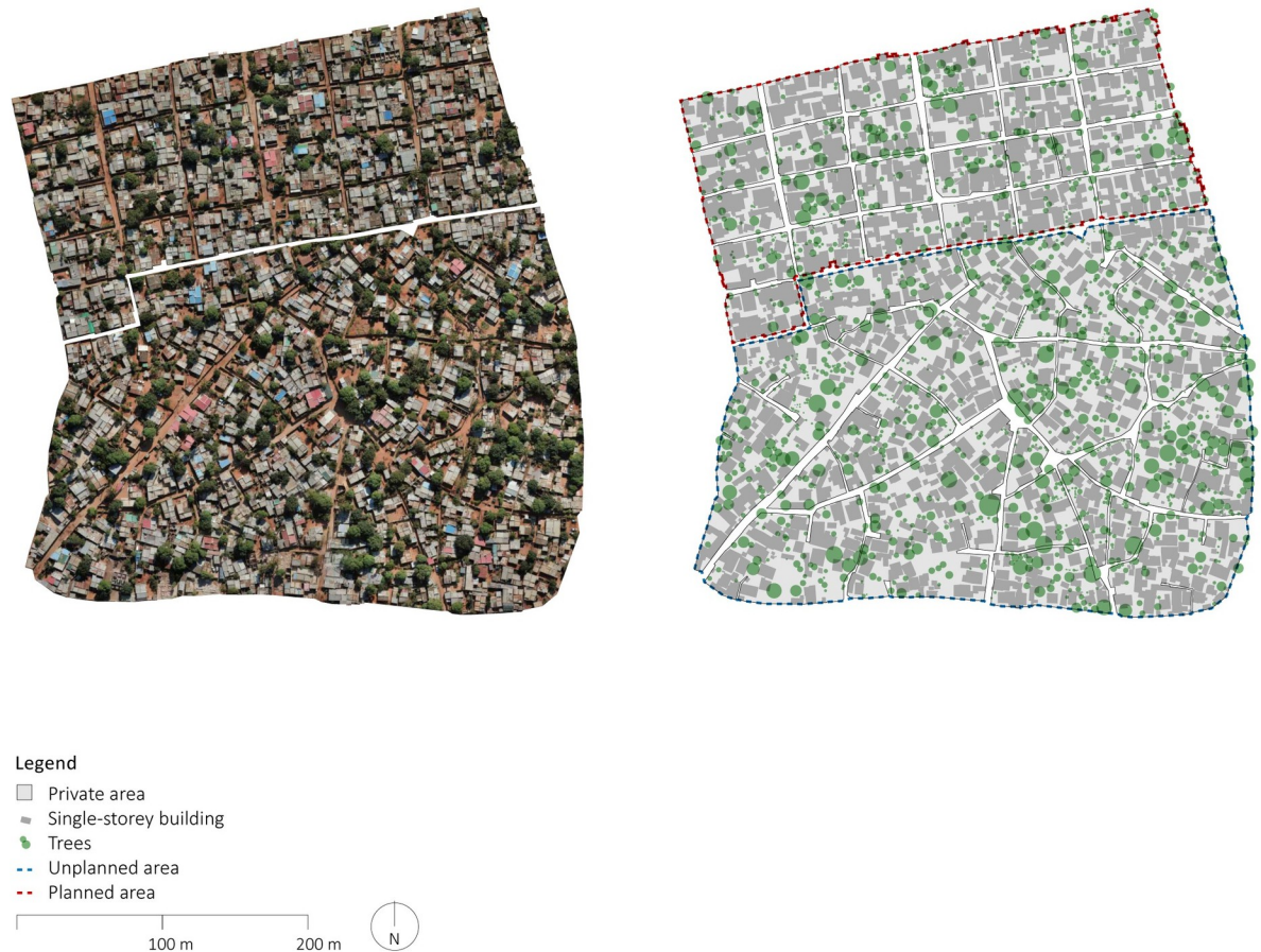
Fig 5. Orthophoto and manually delineated map of Polana Caniço A. The orthophoto was generated using UAVs for systematic collection of photometric data and Pix4D for data processing. The map was created by manually annotating the orthophoto using QGIS and AutoCAD. Source: Johan Mottelson.
