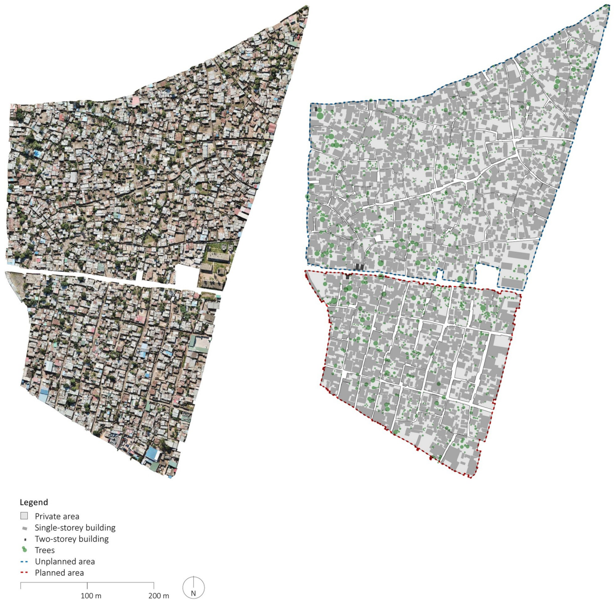
Fig 3. Orthophoto and manually delineated map of Maxaquene A. The orthophoto was generated using UAVs for systematic collection of photometric data and Pix4D for data processing. The map was created by manually annotating the orthophoto using QGIS and AutoCAD. Source: Johan Mottelson.
