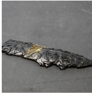
9 Radicant: A 3d-printed biopolymer composite wall paneling system. The panels are composed of interlacing print beads and varying material recipes.
