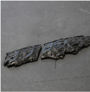
9 Radicant: A 3d-printed biopolymer composite wall paneling system. The panels are composed of interlacing print beads and varying material recipes.
