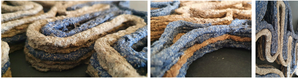
4 (left) Tessellation iterations produced by the agent-based algorithm; (right) final tessellation volumetrically staggered
