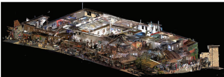
Fig.5: The point-cloud 3D model of Pilavoğlu Han Model is prepared by the laser scanning data in FaroScene by the Project Team.
