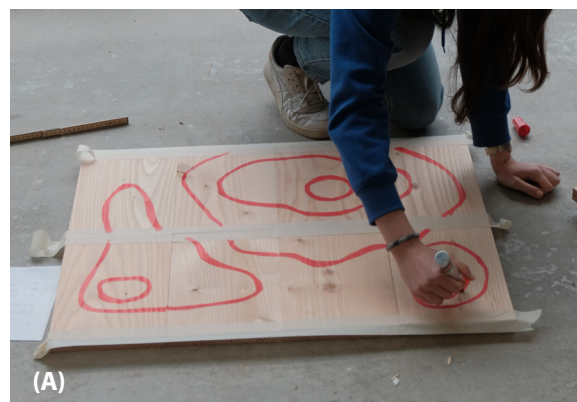
Fig 4.11 A) Robotic programming through drawing, where B) is the milled version; the parameters that control the depth and smoothness, are specified in the software.
