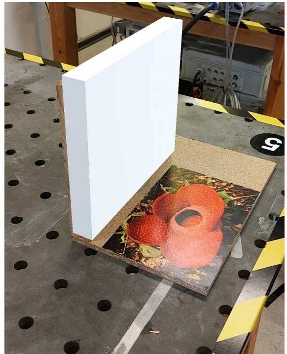
Fig 4.6 An image of the AR pipeline used for the first paper where the object (box) should be positioned on top of a timber physical block based on the floral marker. But as the image highlights, the white block deviates too much from its physical twin.
