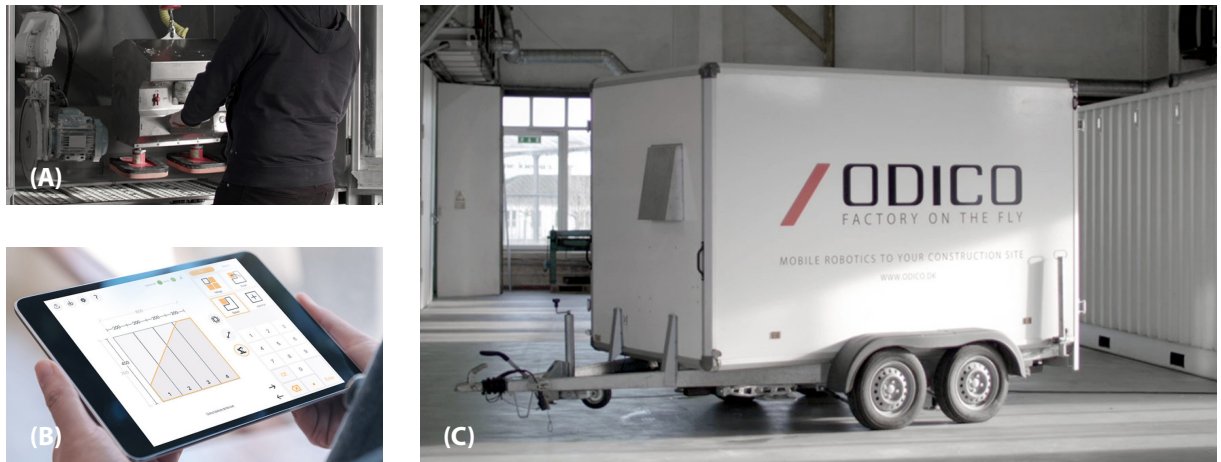
Fig 1.3 A) A paver positioning a pavement stone in the robotic work environment. B) A snapshot of the software which enables pavers to instruct cuts to the robotic unit, and C) the full system, where the robot is positioned within a trailer environment, making it highly transportable.
