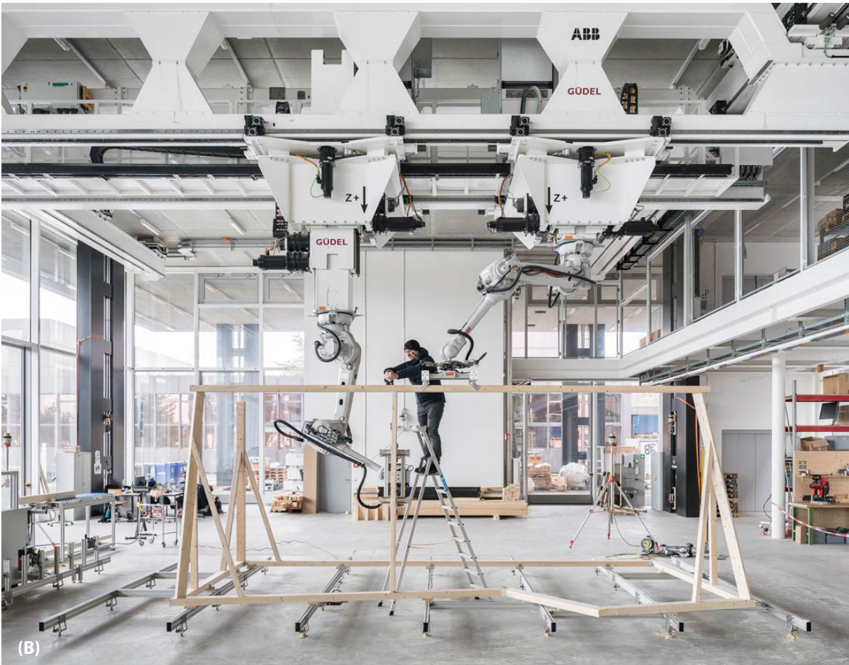
Fig 2.3 A diagram showing the two individual approaches to robotic fabrication. A) Illustrates the ‘fabricator’ approach to robotic fabrication, image from the fabrication of the Landesgartenschau Exhibition Hall, 2014, © ICD/ITKE/IIGS University of Stuttgart. B) illustrates the ‘assembler’ approach from the Spatial Timber Assemblies project, 2018, © NCCR Digital Fabrication / Roman Keller.
