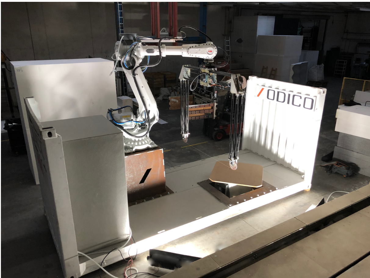
Fig 1.2 A Factory-on-the-Fly system, equipped here for robotic abrasive wire cutting.
