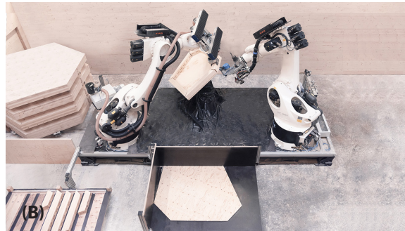
Fig 2.12 A) The TIM framework in its transportation configuration, and B) the TIM framework unpacked and operational in a near-site facility, Germany, 2019, © ICD/ITKE/IIGS University of Stuttgart.
