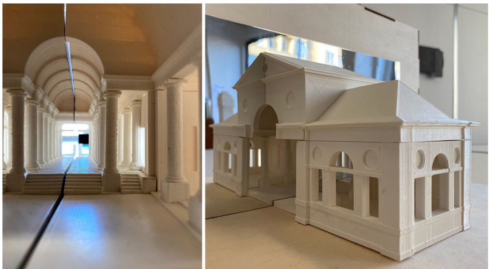
Fig. 04. 3D printing of the accelerated perspective of the small theatre's inner space.
