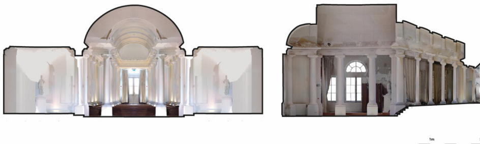
Fig. 01. Transversal and longitudinal section coming from the lasergrammetric survey of the interior space of Seneffe castle's small theatre.
