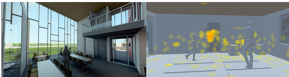
Figure 3 - A 3d rendering from the project (name omitted for peer review) (left) and heatmap showing where users looked when traversing the VR model (right).
