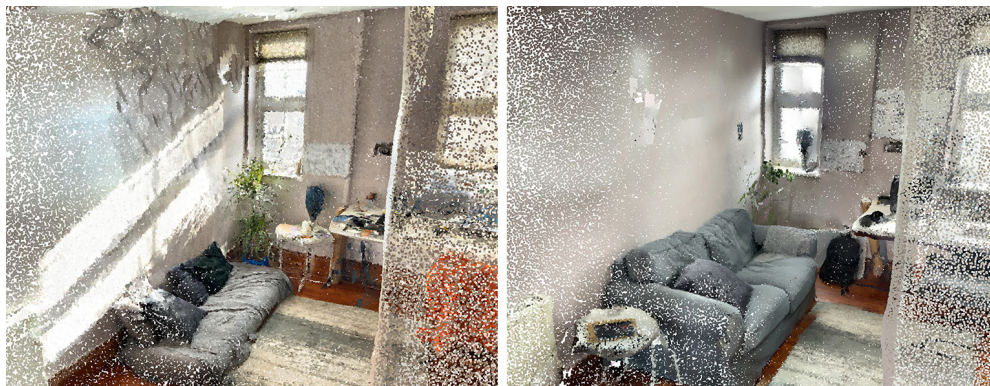
Fig. 01. Visualizations from two 3D scans of the same space with different lightning conditions.
