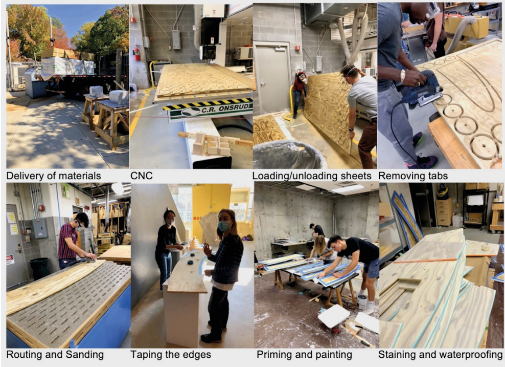
Fig. 08. Fibonacci Nook | Fabrication and Assembly Process
