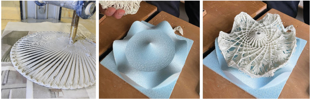
Fig. 04. 3D-printing in porcelain, lasercutted foam and 3D print on foam
