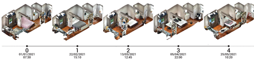
Fig. 07. Visualization of the case study's sequential input data. The resolution of the scans affected the quality and accuracy of the resulting 3D model. Higher resolution scans capture more detail and produce a more accurate representation of the room, while lower resolution scans may miss some small details or produce a less accurate model. The iPhone's LiDAR scanner has a resolution of approximately 1mm, which is sufficient for capturing most of the details in a typical bedroom. However,
