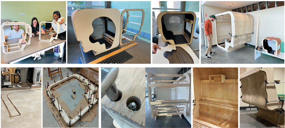
Figure 7 (top row): The development of full-scale construction for structure, envelope, and assembly was based on a 25% reduced scale (3" = 1'-0" scale) physical model.
