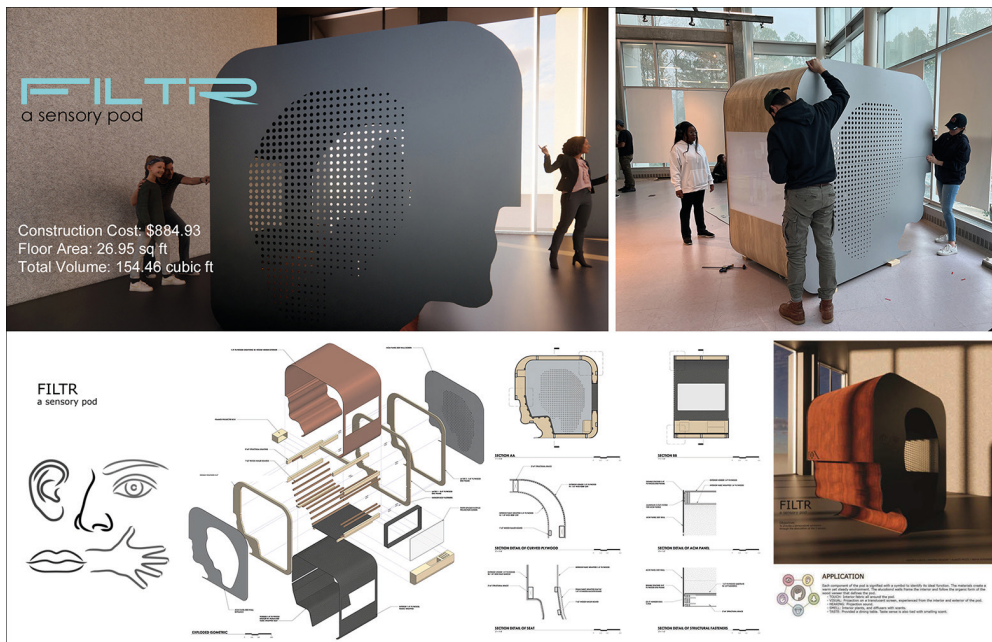
Figure 6: The Sensory Pod proposal with orthographic drawings and a detailed physical model
