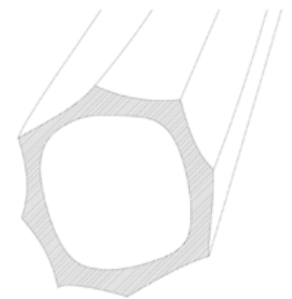
reeds and straw transport water effectively due to their polygonal shape and the surface tension of water
