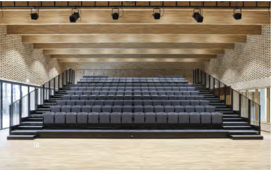
The open, exposed brickwork in the main hall helps to create good acoustics. The hall can be used for many different purposes. A mobile staircase provides seating in the hall for concerts and plays. Photo: Stephane Chalmeau
