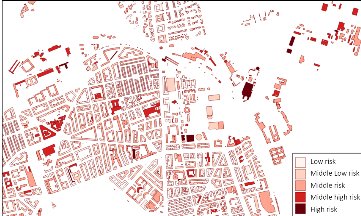
Figure 2. GIS map of the demolition risk of existing buildings in a section of Copenhagen on a graduated color scale. Dark red buildings are at high risk of demolition and therefore need assessment of opportunities to apply circular design strategies, whereas white colored buildings are at low risk of demolition.
