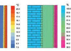
Results from Delphin analysis: scenario: Original wall, air cavity, and wood plate. Left: moisture build up. Right: temperature/heat loss (average over 5 years).
