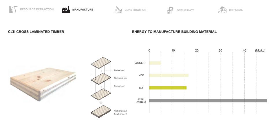
Cross Laminated Timber (CLT) is an engineered wood product made from layers of solid-sawn lumber glued together. Each layer of board, known as a lamella, is orientated perpendicular to the adjacent layers and glued on the wide faces of each board to provide optimum strength. CLT was selected as a building material for the project, after considering its advantages over steel, concrete, and masonry construction in terms of environmental impact.
