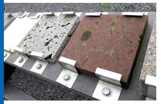
substrate samples to test for lichen growth at DTU
