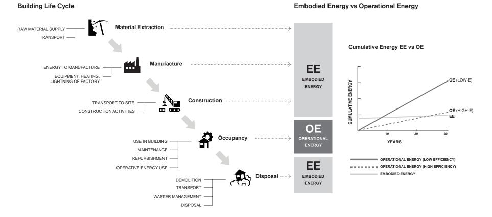
While most sustainable design strategies have been focusing on operational energy (the energy used for occupancy and maintenance), the embodied energy (the energy embodied in the material extraction, manufacture, and transport of building components, and the
