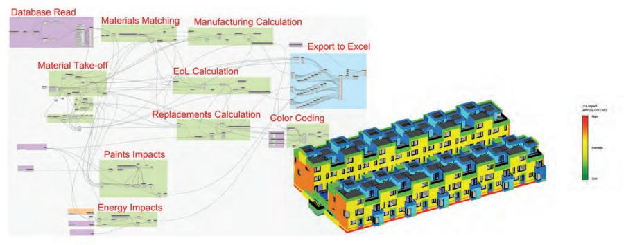
In this work, tools are built to couple logical processes and routines, and to bridge the existing simulation and calculation tools that are necessary to generate relevant feedback for the designers. Vandkunsten's project Havnevigen is analyzed with an LCA tool that utilizes the BIM7AA encoding system as well as the Ökobau LCA database.
