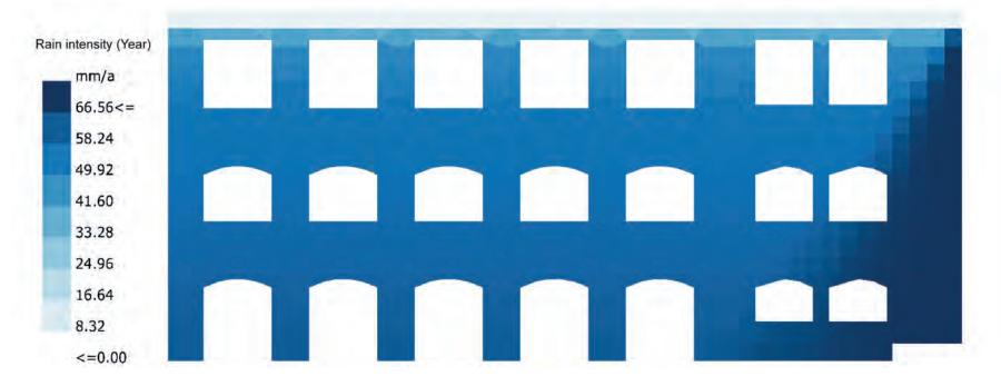
Some tools are built from scratch. When tools are not available elsewhere, we use existing research papers from various narrow fields and implement methods, algorithms, and procedures as code. Above is a tool that simulates annual driving rain on walls.
