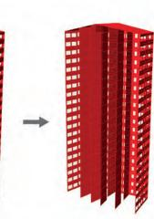
HORIZONTAL DISPLACEMENT Max. allowed: H / 500 - 142.4 mm Remember: the load cases that should be checked are the SLS characteristic combinations If the criteria is not fulfilled: - Increase wall thickness - Reduce wall openings -Add internal shear walls Load case5 - 319.99 mm - NOT SATISFIED
