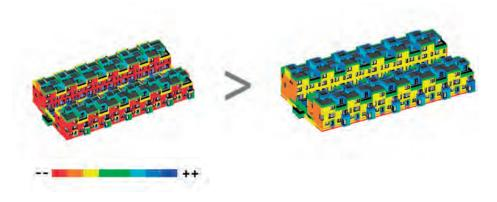
Fig 1: Visualization of impact category "global warming potential" for two options of a building design regarding materiality. Graphics are generated with Aeforos in Revit.
