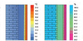
Results from Delphin analysis: scenario: Original wall, air cavity, insulation, and wood plate. Left: moisture build up. Right: temperature/heat loss (average over 5 years).
