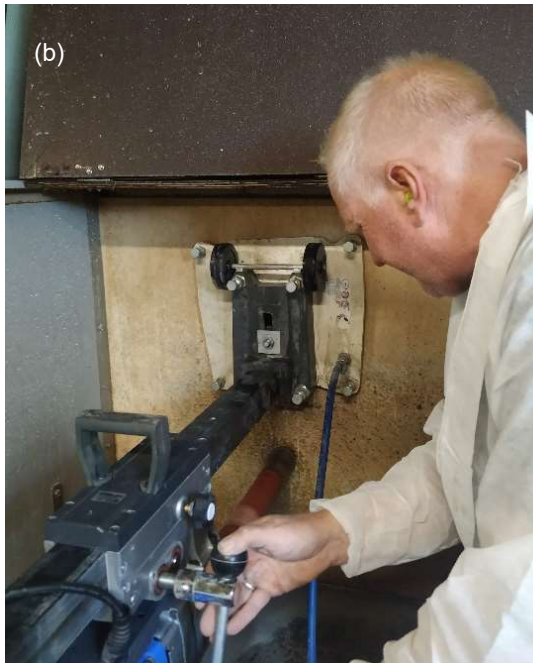
Figure 1: (a) The core drilling machine, (B) the core drilling machine during sampling at a wall, and (c) the wall in Stable A after sampling,
