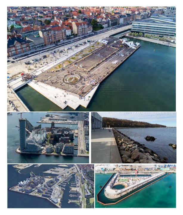
Figure 70. (Top image) A photo of the reclaimed land recreational area of the waterfront of Aarhus. It is largely made up of the impermeable surface of asphalt and concrete (heat island effect in summer); it makes very little consideration for the engagement of coastal ecosystems nor any buffer space for excess water. Image credit: Kultur Aarhus and Dennis Borup Jakobsen.
