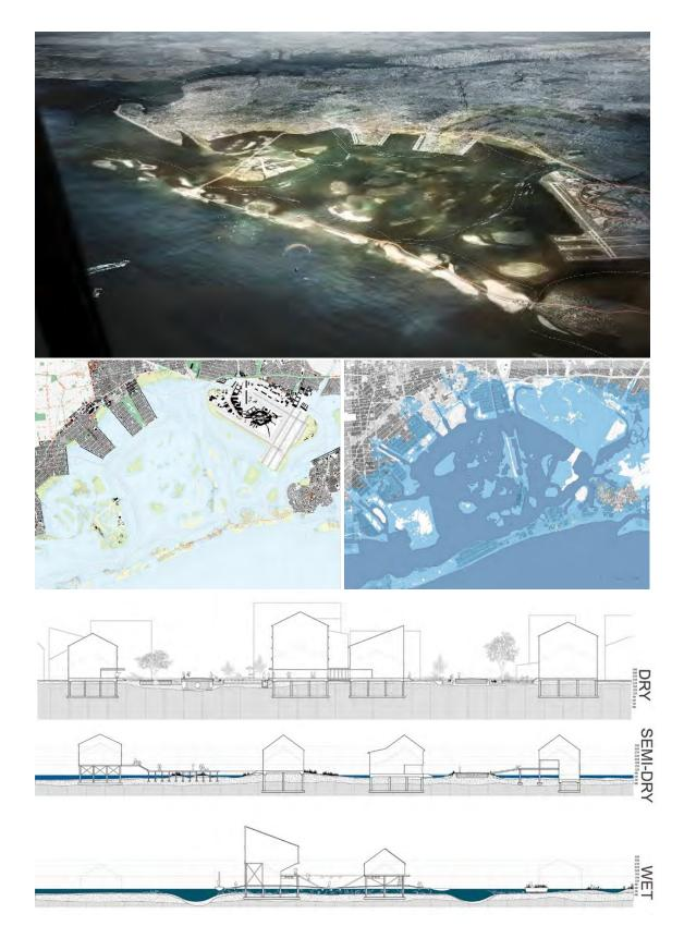
Figure 84. Project by Rafi Segal A+U and DLand Studios (Susannah Drake) – "Bight: Coastal Urbanism" in the Tri-State, USA. This project aims to replace the hard edge that segregates the city and sea with a new "landscape economic zone — a buffer that allows land and water to commingle, creating new spaces for habitation, conservation, work, and play. This project is an example of long-term retreat as part of the coastal adaptation strategy" (DLand Studio, n.d.).
