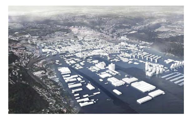
Figure 6. (Top image) Vejle faces several water issues from the fjord/sea in the form of storm surges (exacerbated by sea-level rise), rise in groundwater and the water coming down from the hills due to its location at the bottom of the river valley where the two rivers/streams meet. Image credit: Vejle Municipality (2020a).
