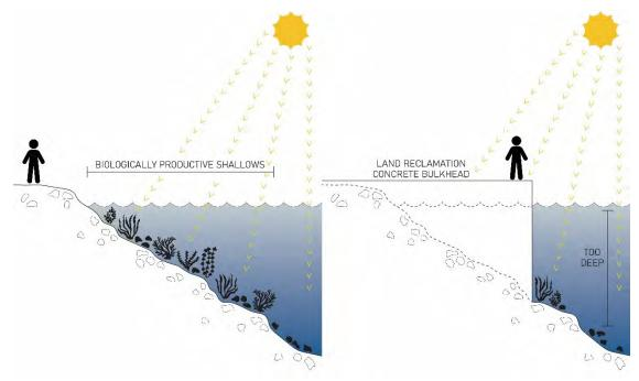
Figure 11. (Top Left image) Illustration of how coastal ecosystems such as seaweed depends on a certain depth below the sea (depending on water clarity) to access sunlight for photosynthesis and is sensitive to thermal stress (Dahl et al., 2003; Harley et al., 2012). Hence, many coastal ecosystems thrive at an ideal depth below sea level, which land reclamation projects have replaced (the shallow areas). Image credit: Dahl et al., (2003).
