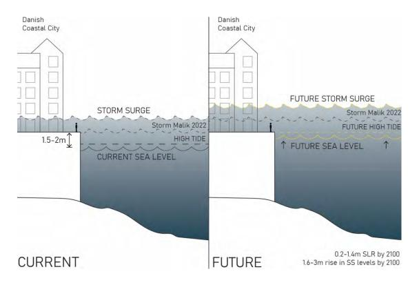
Figure 56. A diagram showing the relationship between SLR and SS in its impact on inundating coastal cities in Denmark with Storm surge range for Little Belt Sea (Lillebælt where Vejle is). SLR alone will not cause inundation of coastal cities (even in a worst-case scenario), but SLR coupled with frequent and more intense SS has the potential to wreak havoc in a worst-case scenario situation. Image credit: Soo Ryu and Agnes Jarmund.
