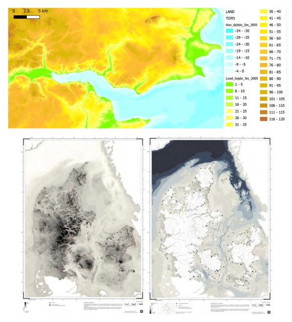
Figure 37. (Top image) Topographic and bathymetric data of Vejle fjord. The different colour gradation represents different heights above and below the current average sea level. This type of topobathy map is useful when engaging with a site that concerns the boundary between land and sea.
