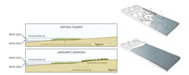
Figure 59. (Left image) Coastal nature is able to migrate landward as sea level rise, preventing coastal squeeze. (Right image) Diagram showing an urban scenario where a rise in sea level drowns the existing salt marsh in front of cities due to the creation of a dike to protect the city from flooding. Image credit for both images: COWI and Arkitema, 2021 (Ebbensgaard et al., 2022b).
