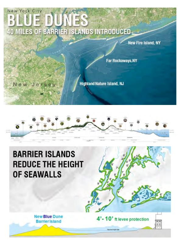
Figure 87. A hybrid approach where barrier islands out in the deeper waters are created to host dynamic ecologies to protect from storm surges in combination with levee protection inland. "Blue Dunes" by WXY Architecture + Urban Design and West 8 for NYC, USA (Keenan and Weisz, 2020). Image credit: Rebuild by Design (n.d.), WXY Architecture + Urban Design and West 8.
