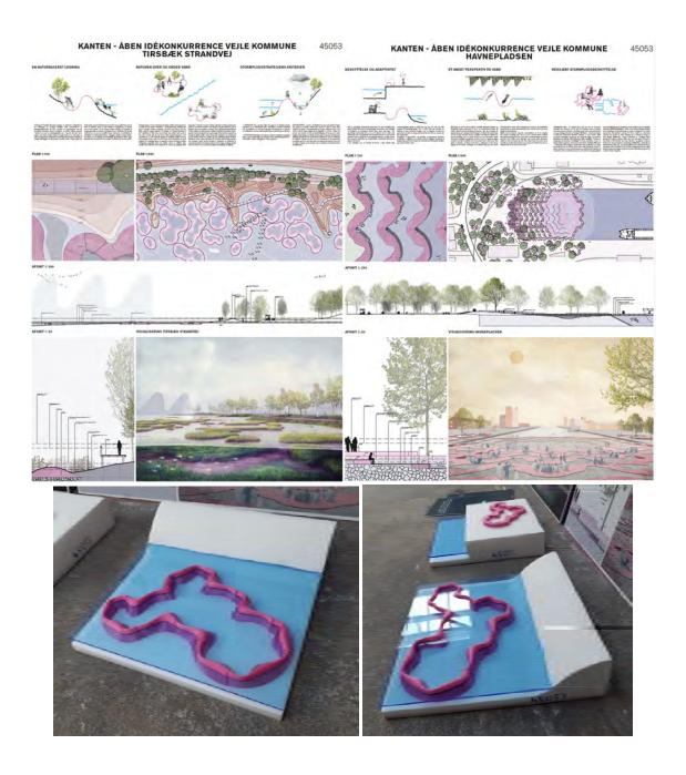
Figure 131. Images of the final A1 panels for each zone and the physical models of their entry. The undulating pink surfaces are for marine life to attach to in the water. Image credit: Vejle Municipality and SUPERFLEX/Baldios. (photos of the physical models taken by the author on 13/08/20). (Extracted from Kumu Multiscalar map – Kanten/The Edge scale node).
