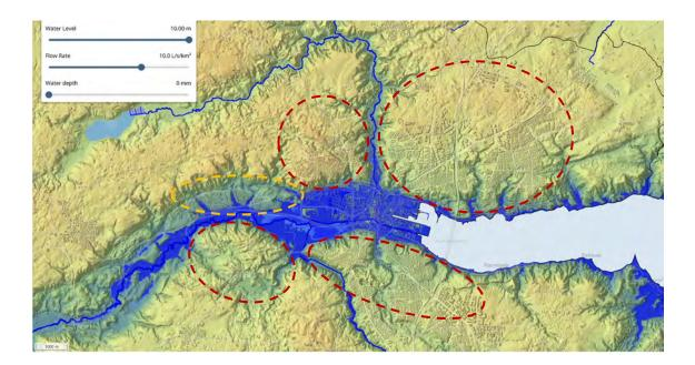
Figure 173. The future scenario of 10m SLR in Vejle, where the entire river valley is inundated (shown in blue). The surrounding suburbs on top of the river valley are safe up to 21m of SLR (red outline), guaranteeing protection from inundation. A potential area for a new harbourfront/waterfront on land would need to be 4km back from the current Fjordbyen (outline in yellow). Map credit: SKALGO (n.d.).
