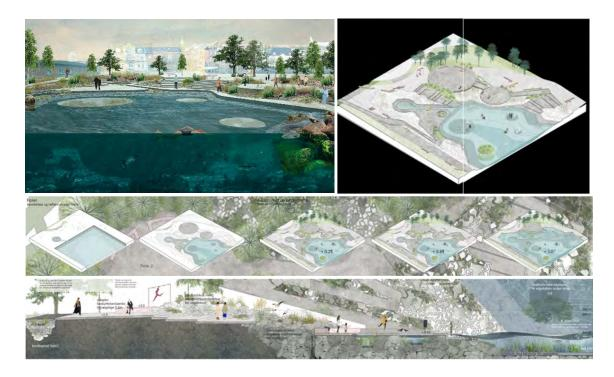
Figure 118. Visualisations for the Urban Zone. The intention of the design is that as the water level rises, the stone landscape out into the water also grows with time. Various platforms, benches and staircases allow the meeting between human and nonhuman subjects. Image credit: Vejle Municipality, Josephine Philipsen, Luisa Brando, and Andres Hernandez. (Extracted from Kumu Multiscalar map – Kanten/The Edge scale node).
