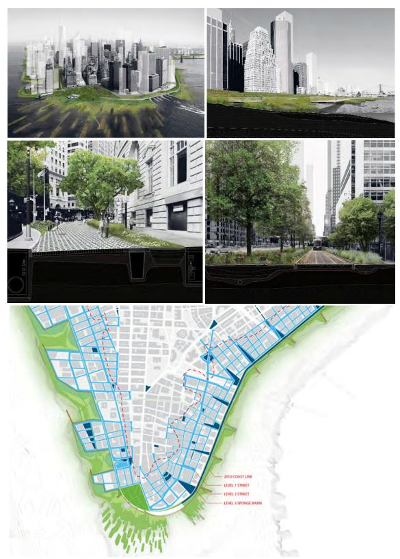
Figure 88. A hybrid approach proposal by DLand Studios and ARO is called "A New Urban Ground." The proposals refurbish existing hard infrastructure systems, including perimeter wetlands, a raised edge, and absorptive sponge slips paired with new upland street infrastructure systems, protecting the island from flooding in the event of a large storm (DLand Studio and Sasaki, 2022). Image credit: Dland Studio.
