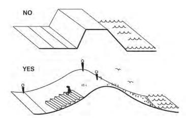
Figure 69. (First and second row of images) The Blue Line signifies a small departure from the previous B-A-U of land-reclaimed harbour constructions, where the traditional edge conditions did not consider any form of landscaping or seascaping (nor accessibility or recreation). Image credit: C.F. Møller Architects (2019).
