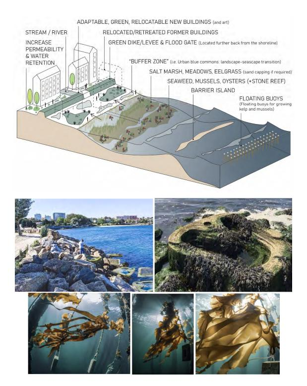
Figure 86. (Top image) An example of a hybrid approach with growing interest and evidence supports the combination of natural infrastructure, built infrastructure and retreat strategy to enhance coastal resilience. Image credit: Redrawn and redesigned diagram by Soo Ryu and Agnes Varmund (based on Sutton-Grier et al. (2015)).
