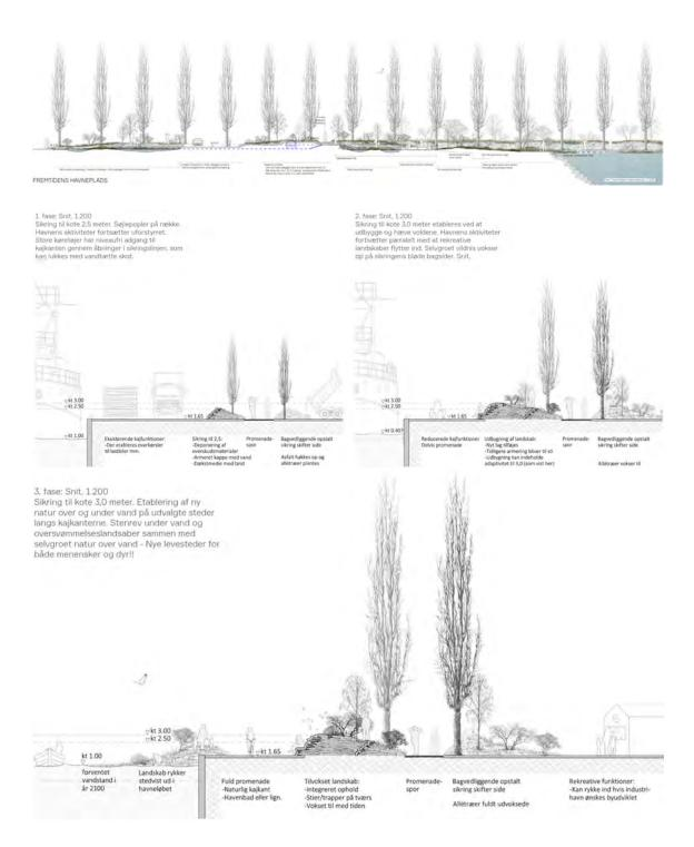
Figure 125. The section of the Urban Zone, where the landscaped embankments made of surplus construction materials provide coastal protection by growing with time while landscaping also envelops these concrete mounds. Image credit: Vejle Municipality, Jonathan Houser and Jonas Lambert. (Extracted from Kumu Multiscalar map – Kanten/The Edge scale node).
