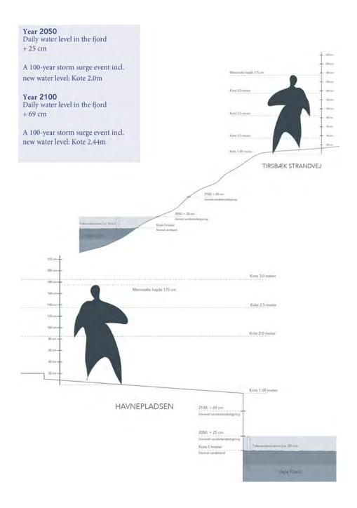
Figure 108. "Kote" (elevation) level o corresponds approximately to the current normal water level in the fjord (tidal variation of approximately 50cm). The Edge/Kanten protection levels are 2.5m for protection and 3.0m for adaptation (Vejle Municipality, 2020a). Image credit: Vejle Municipality (2020a, n.d.). (Extracted from Kumu Multiscalar map – Kanten/The Edge scale node).
