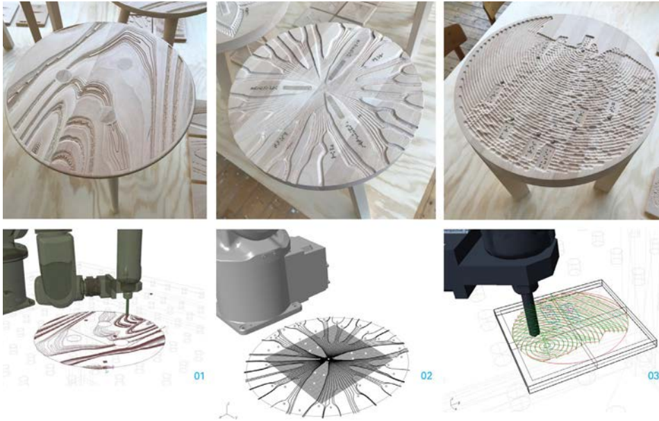
Project Framework: stool variations. P1 'Woodgrain' transfers wood grains and available surface patterns into tactility (01), P3 'Flowers and Fluids' discusses randomised order and directionality (02). P5 'Spatial Map' combining image source for centric wave relative to location (03).
