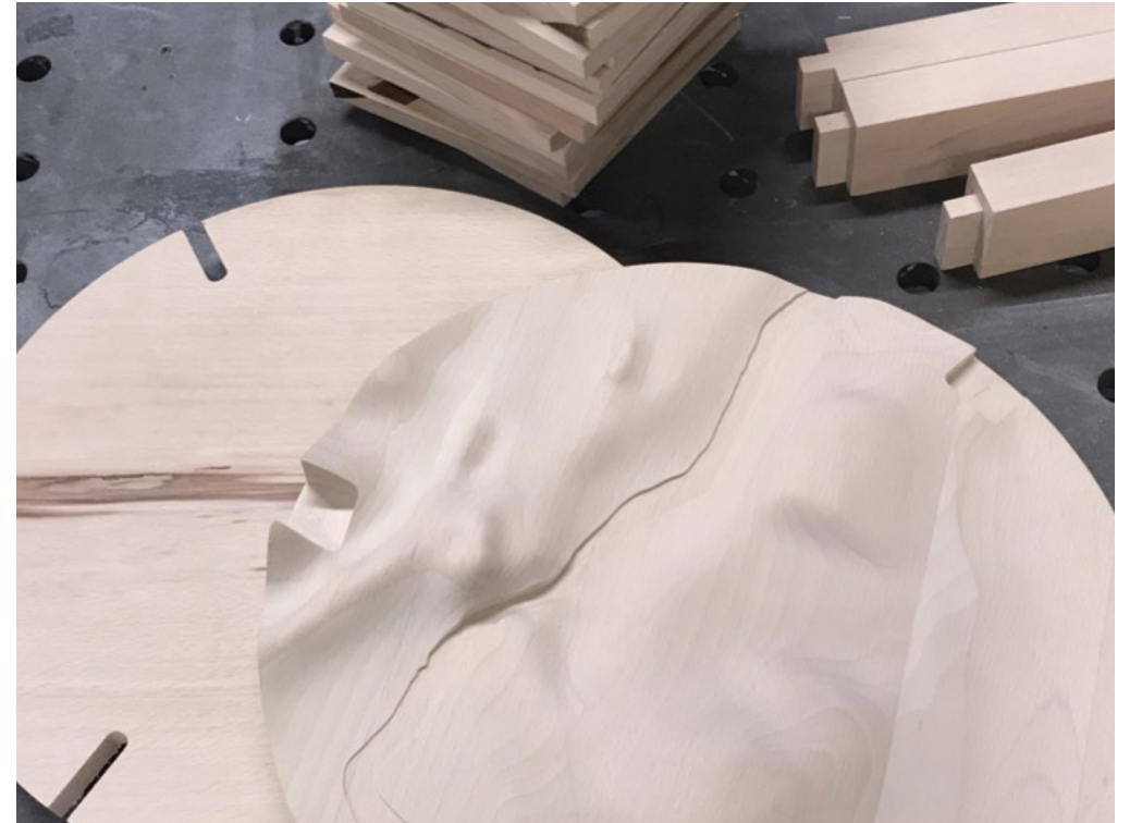
Multiple Tooling processes from routing deep topography in stool surface through 5axis CNCing, robotic milling and manually embedding Braille.
