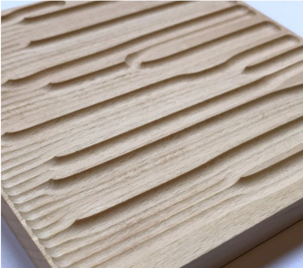
Script 3 based surface treatment studying the appearance and readability of a directional flow, with surfaces left for Braille text inserts. (150x150mm, beech)
