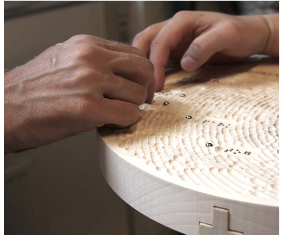
Manual inserts of ballbearings into robotically milled surface as a text for Braille readers.
