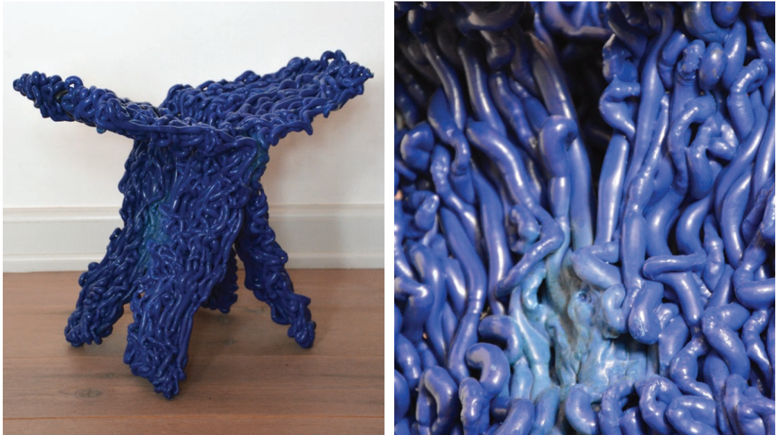
Figure 2.3.18 - Interpretation of Sori Yanagi's Butterfly Chair, from robotic extrusion of recycled polypropylene
