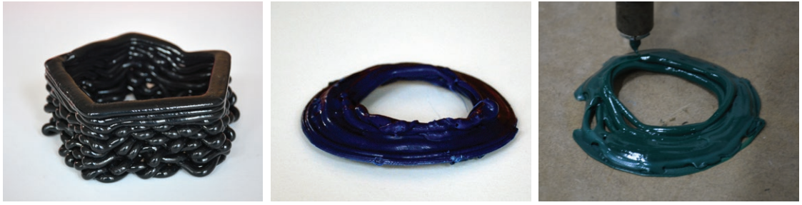
Figure 2.3.16 - Test Prints of Polystyrene, Polypropylene, and High Density Polyethylene
