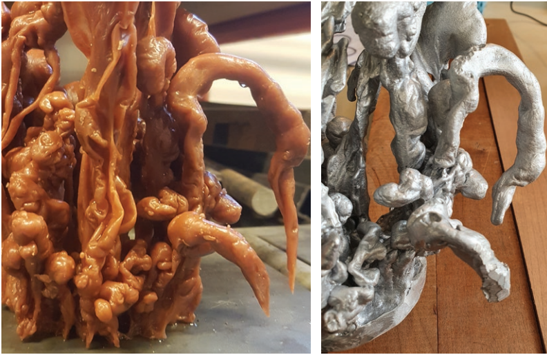
Figure 2.3.15 - Fluid wax deposition, and aluminum casting of wax object
