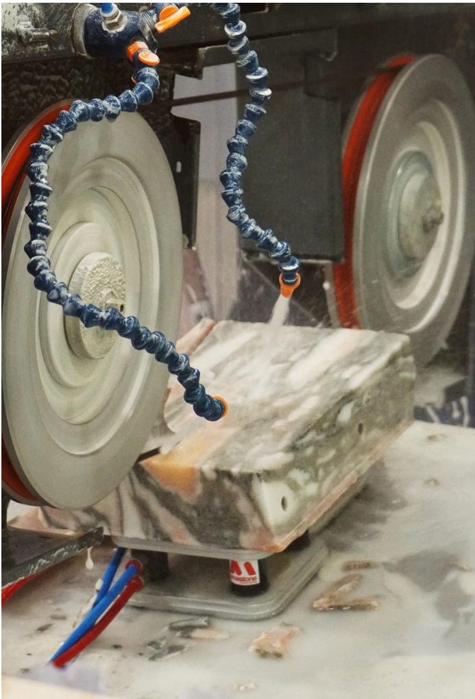
Clockwise from upper-left: Robotic drilling to split and book-match marble for Column Drilled holes ready for analog splitting of marble for Column Edge articulation to create a block of marble for Wall Ruled surface cutting of marble block to reveal translucency in Wall
