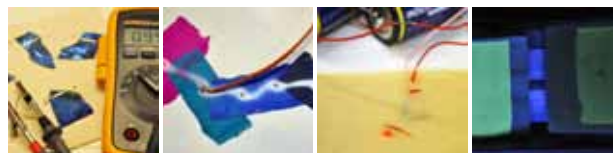
Figure 3: Representations of the preliminary experiments. From left: solar cells, thermochromic print, LEDs, phosphorescent print (photo: Karen Marie Hasling).
