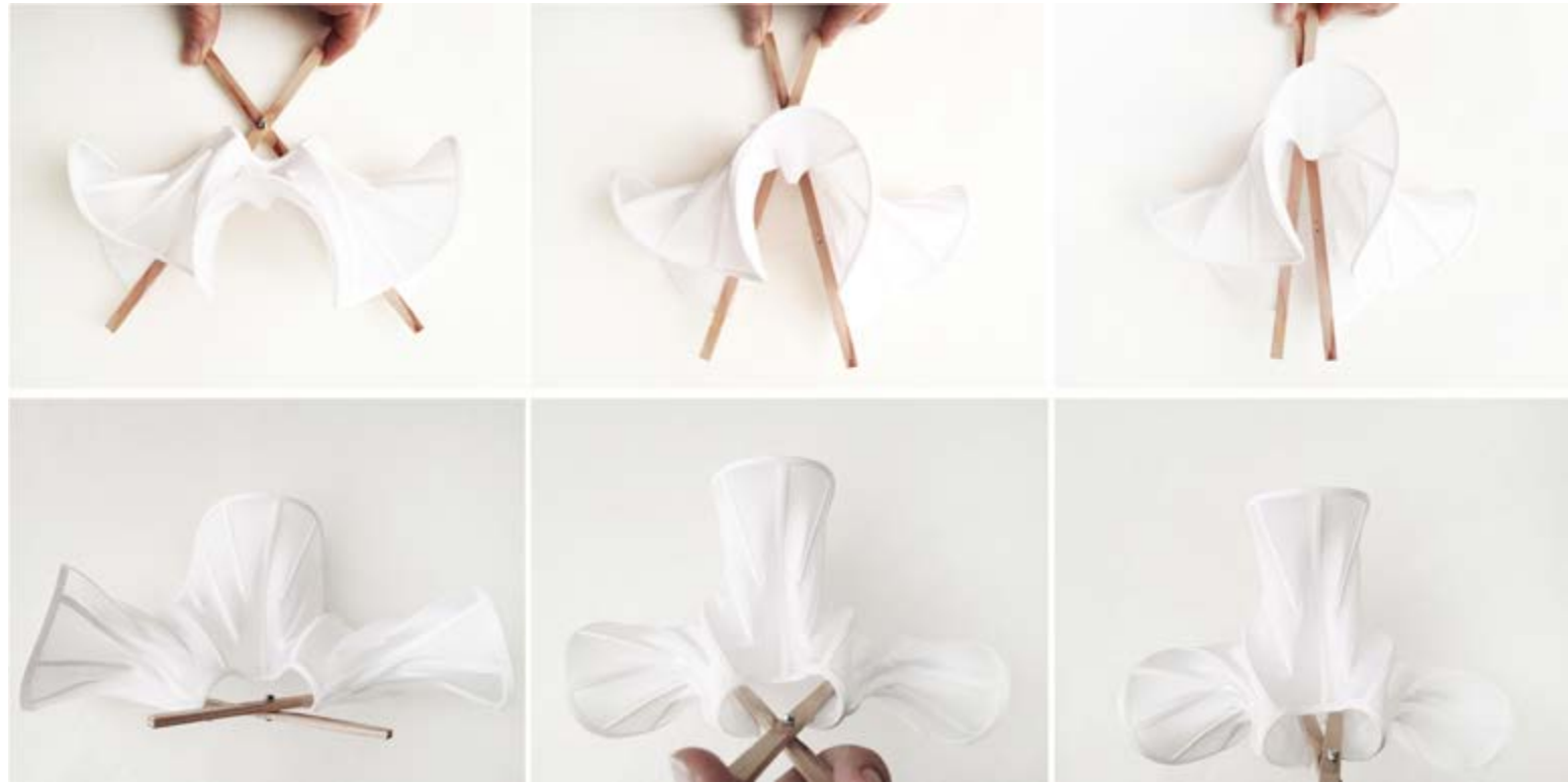
FIGURE 11. Studies of the movement of a textile module with ribs and enclosed boundary, attached to a wooden structure: top view (upper row), side view (lower row)
