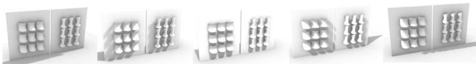
FIGURE 08. Sun path analysis of open and closed modules facing south, located in Berlin, Germany on July the 17th at the following times: 10:00 AM, 12 AM, 3 PM and 5 PM.
