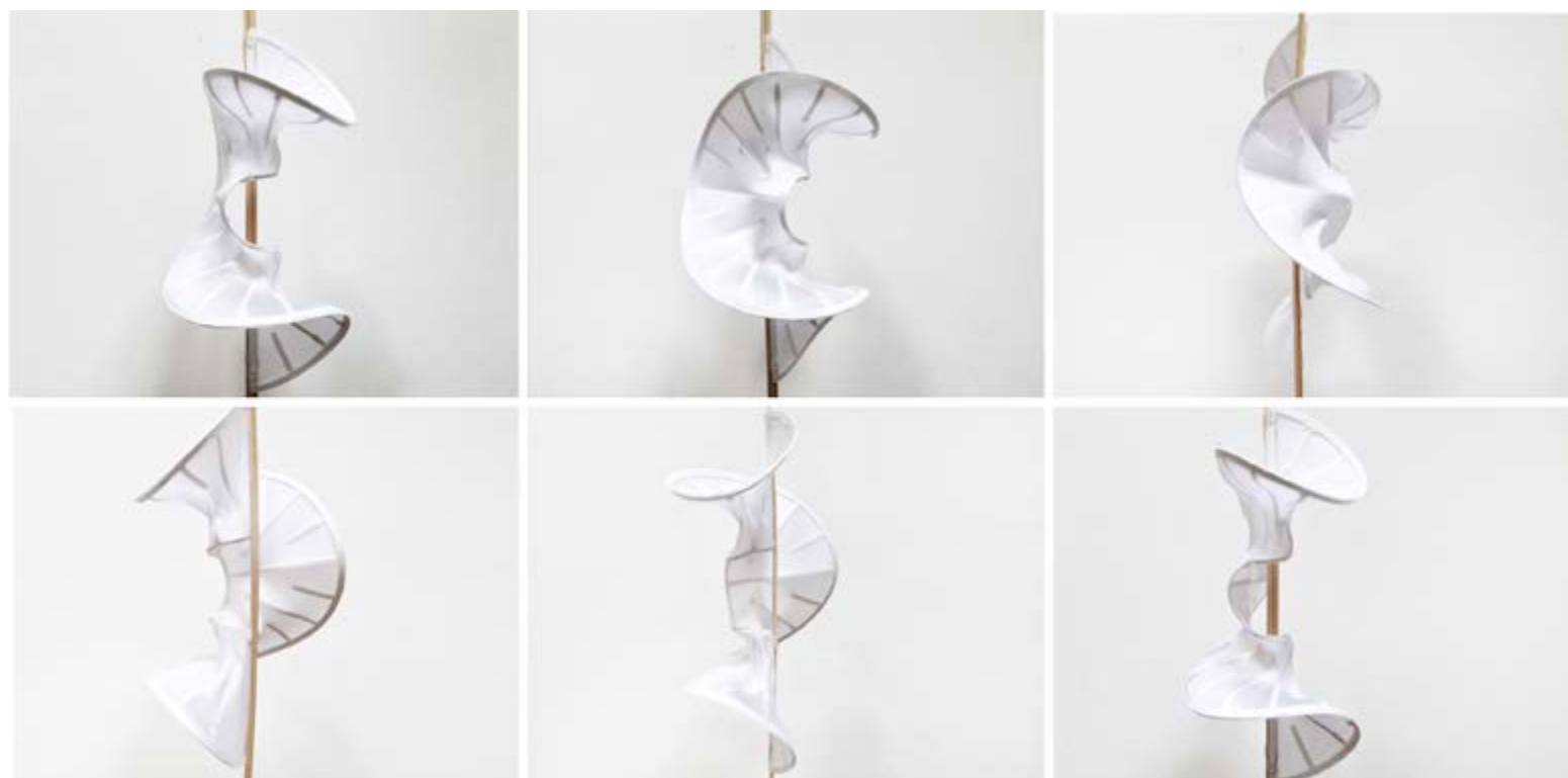
FIGURE 12. Single textile module with ribs and enclosed boundary, attached to a wooden support and rotated along its vertical axis.
