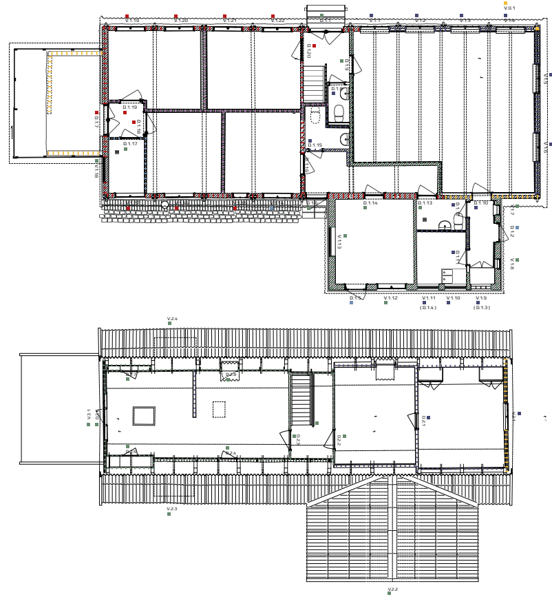
Above, figure 12: Historical building changes over time. The colours on walls, doors and windows indicate how old they are – the red ones are the original from 1887, the orange are extensions from about 1895, the green from after 1916, the blue ones from after 1947, indigo from 1967, and purple is 1970s remodellings.
