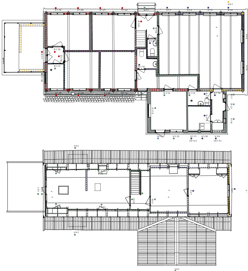
Above, figure 12: Historical building changes over time. The colours on walls, doors and windows indicate how old they are – the red ones are the original from 1887, the orange are extensions from about 1895, the green from after 1916, the blue ones from after 1947, indigo from 1967, and purple is 1970s remodelings.
