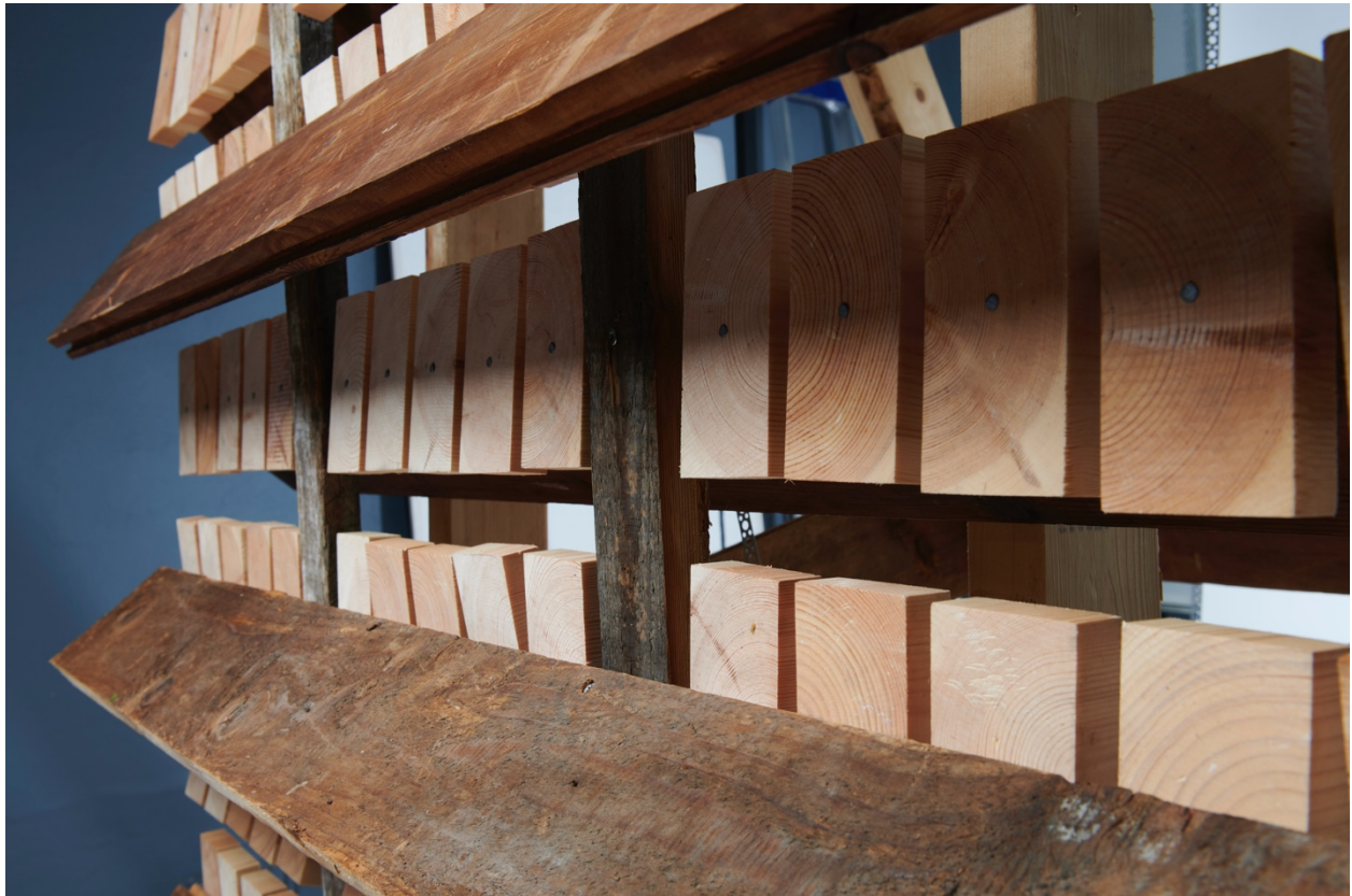
Figure 4: Combining small and long timber elements, close-up
