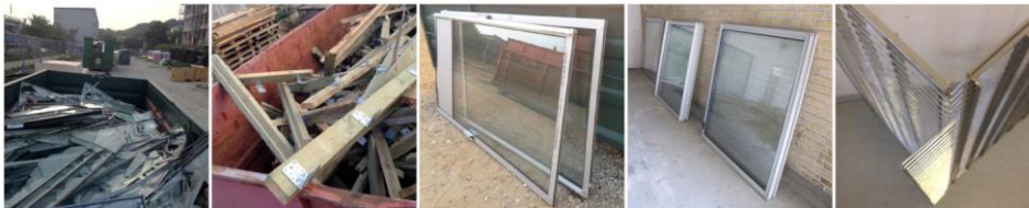
Figure 3: Examples of building waste found locally: window glass, construction timber, aluminium doors and windows, and chromed shelves. Photos Vestergaard.
