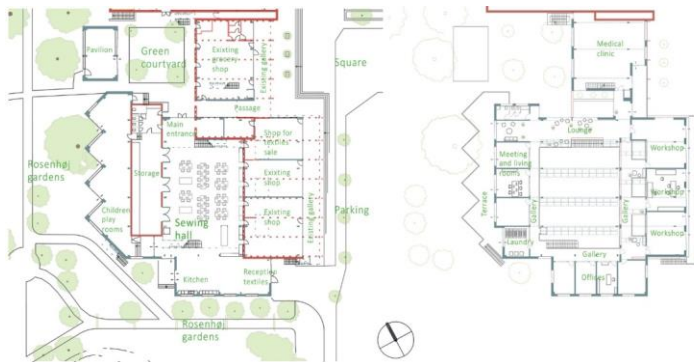
Figure 7: Ground floor and first floor plans of the project. The existing construction is shown in red colour and the new additions in grey colour. Illustration Martín Jiménez.
