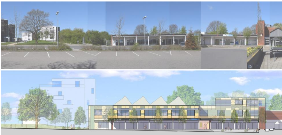
Figure 9: Upper picture: Shopping Centre as it looks before the transformation. Lower picture: transformation of the case project, where the façade is created as an assemblage of the existing wooden portico in combination with the façade expression created with reused steel plates in a modular surface design articulated by the plate's two colors. Illustrations Martín Jiménez.
