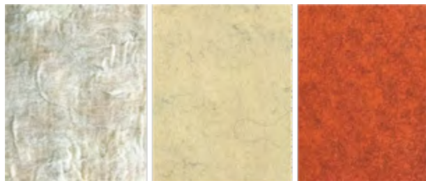
Figure 1: Various felt surfaces. From left to right: wet felting by hand, machine felting, automated felting.
