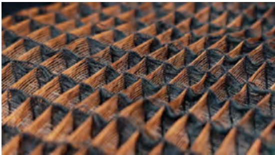
Figure 12 Copper and cotton yarn floats in a waffle weave
