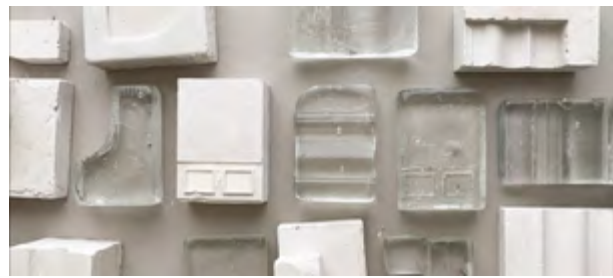
Figure 6: Fragment models in plaster and glass, scales 1:1, 1:5, 1:10, and 1:20. Photo: Liv Sofia Engelbrecht Dannevang.
