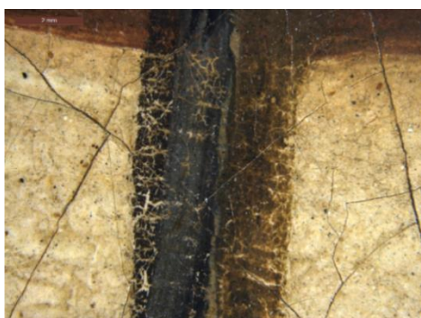
Fig. 5.14 Micrograph of drying cracks in the string around the neck of Battier KMS3634 .
