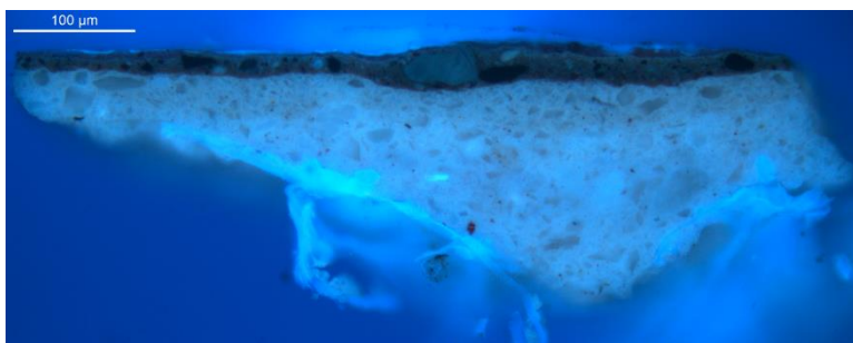
Fig. 8.6 UVa image presenting fluorescence beneath the ground layer in the cross-section of J.Moltke SV5 seeming, on first look, to indicate the use of a sizing layer. However, the fluorescence is due to the canvas fibres.
