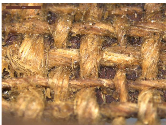
Fig. 8.3 Detail image of the reverse of the canvas of Clemens KMS396 . The red ground layer sits flat over the interstices in the canvas, suggesting either a film-like sizing layer prohibited extrusion or that the ground material was very viscous when applied.
