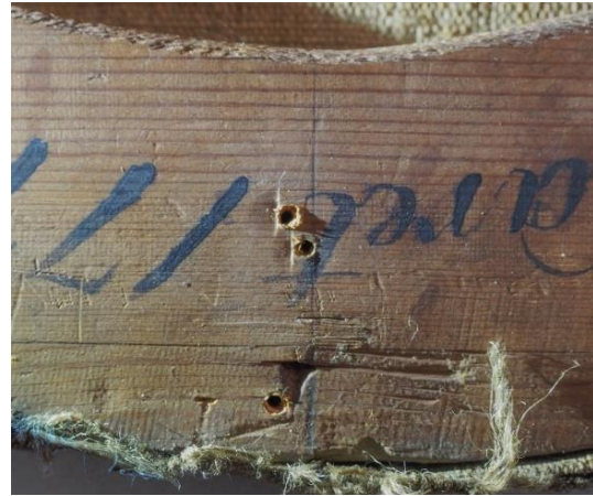
Fig. 6.10 Detail of the central lower member of Hauch KMS349 displaying rippling from a hand plane and a pencil line indication of the major axis.
