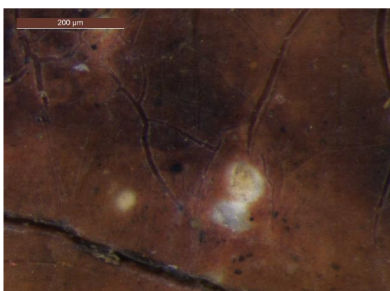
Fig. 5.22 Micrograph of the paint surface of Bagge KMS1115 displaying lead-soap protrusions.
