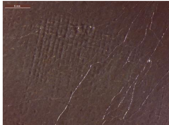
Fig. 5.3 Marks in the paint surface of Holm KMS1766 , likely originating from the hot iron during lining treatment.
