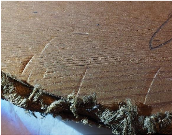
Fig. 6.9 The wooden surface of the original strainer of Buchwaldt SV3 showing deep indentations running parallel to the wood grain likely from a tothing plane. Indentations from the use of stretching pliers are visible along the edge.
