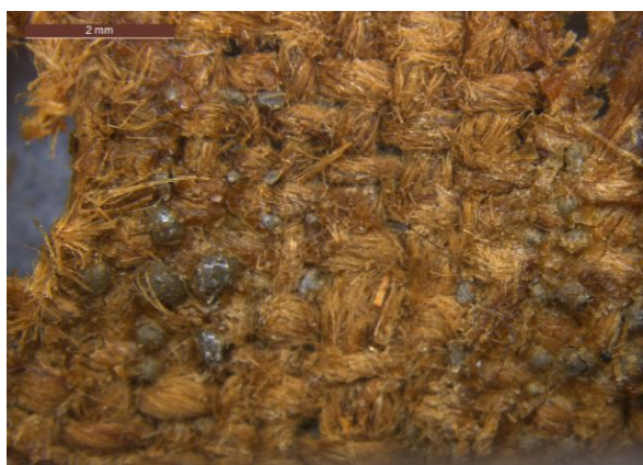
Fig. 8.2 Detail image of the reverse of the tacking margin of Self-portrait KMS3990 displaying protruding ground material consisting of the lower grey layer of the double ground.
