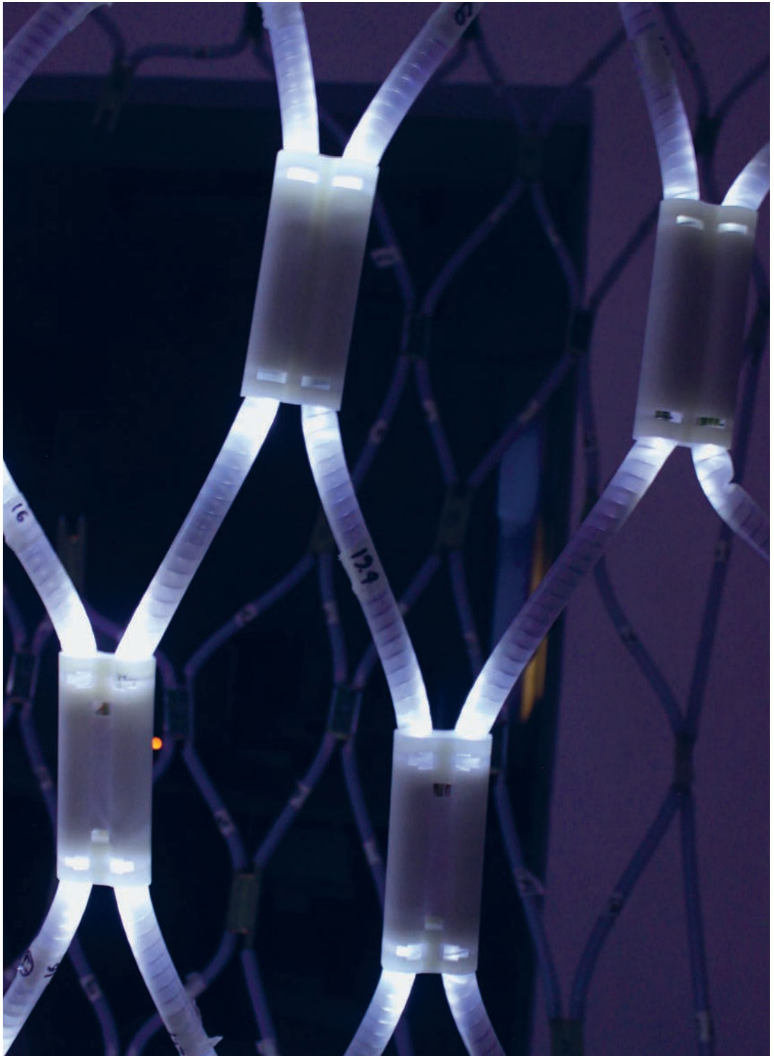
[123] Testing of the 3D-printed housing of the nodes – “on” condition
