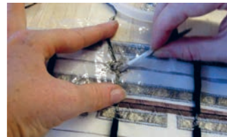
[11] Stitching of low-resistance conductive thread to connect to the PCB (Image Source: Berzowska & Bromley 2007)
