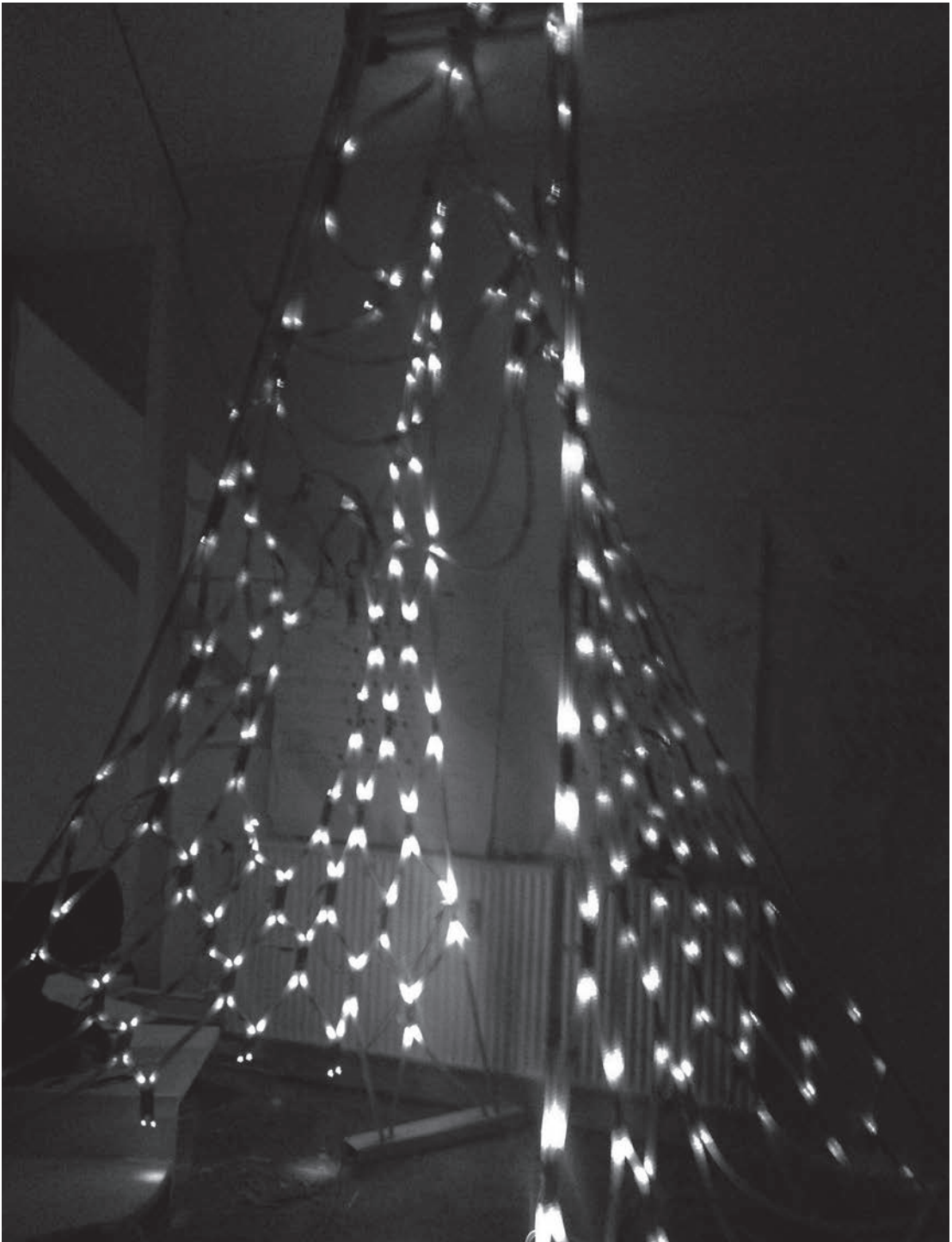
[141] Displaying how the position of the power source is significant for the flow of power and control. When considering the layer towards the street, the gradient reveals that the power source is positioned towards the wall, as the light intensity falls towards the space - view 4
