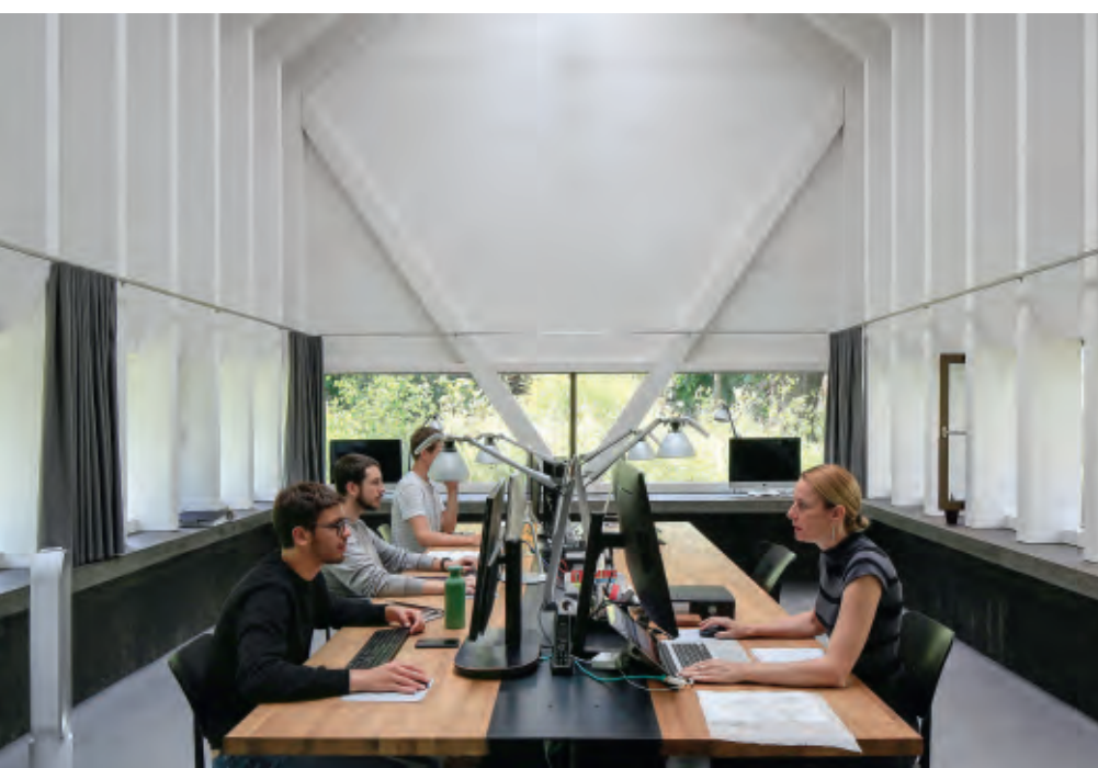
Access to the building is via the ground floor, part of which is below ground and which houses a drawing atelier. The interior has a beautiful and distinctive timber-frame construction, painted in matt, semi-transparent white paint.
