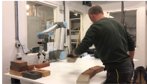
Figure 9 Interaction with Robot : idle robot while mason in working; robot active; brick handover
