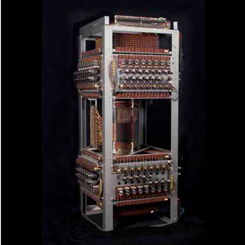
Whirlwind Computer Core Memory Unit
