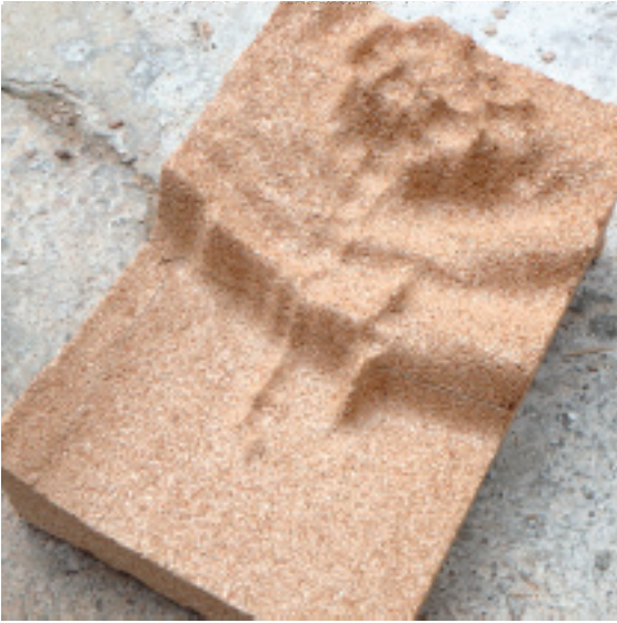
CNC-milling in Ceraform to explore the material and the glass' interaction
