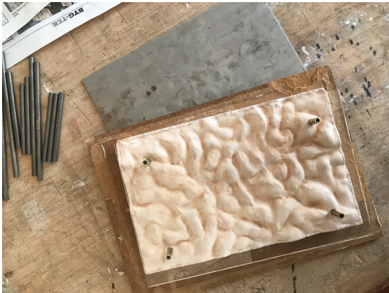
The plaster casted print with the glass on top before the slumping process.
