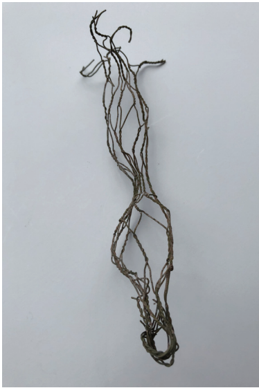
Chicken wire after repeated use and the imprint on the glass surface
