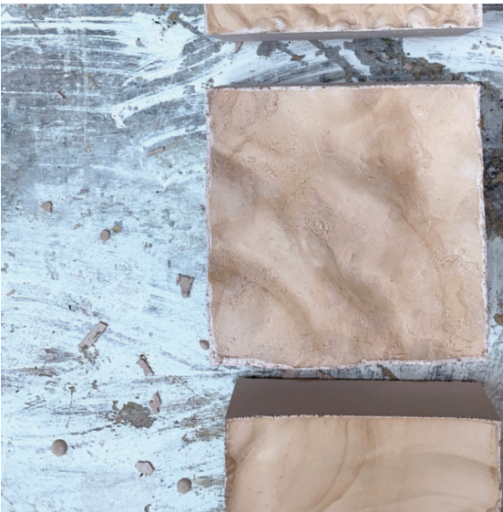
Plaster cast with has to dry and calssine at about 600 degrees.
