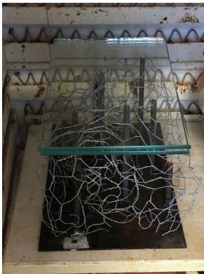
Experiment 09 - Chicken wire on steel bars layers in ceramic oven. Mould and glass become one.
