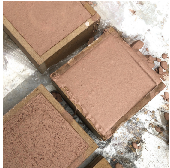
Casting with two part rock cast, one part flint, one part firebrick
