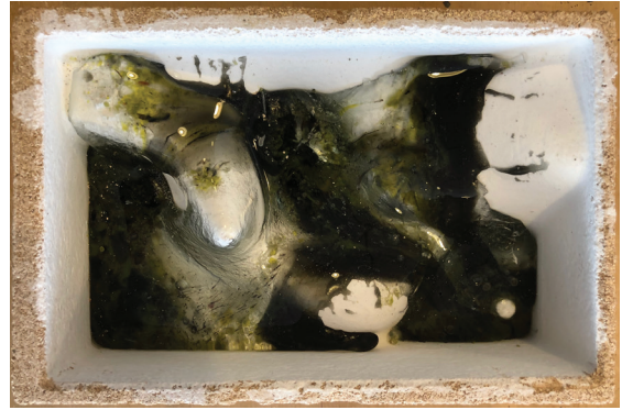
Experiment 06 - CNC mould, after getting into the ceramic oven.
