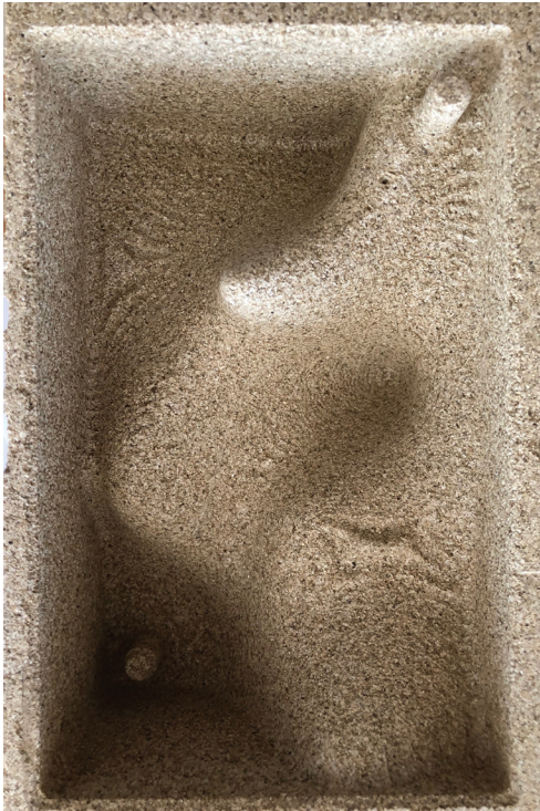
Experiment 04 - CNC mould, the tool lines are very clear and the glass will adapt to the shape.
