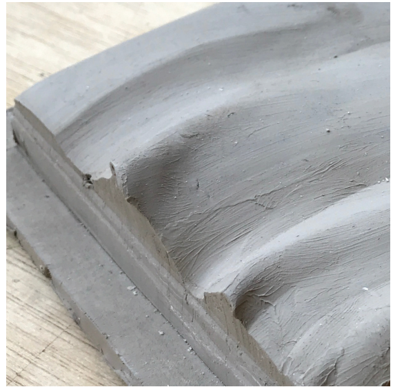
Clay surface before the negative shape will be formed in plaster.
