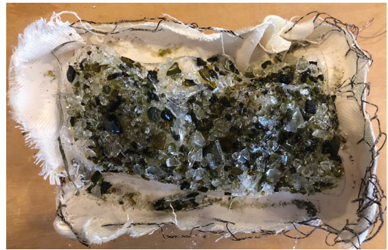
Experiment 02- Fabric mould after getting into the glass oven. Same technique as experiment 6, but the different temperature gives a very different outcome.
