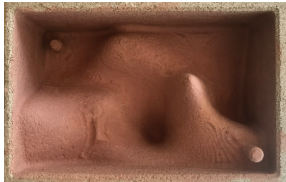
Experiment 04 - The glass sticks to the form unless the form is coated with glass slip.
