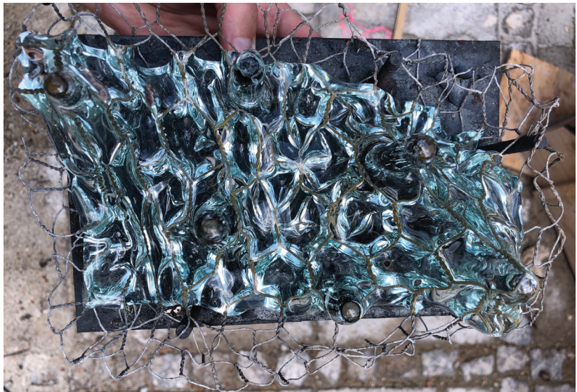
Experiment 02- Fabric mould after getting into the glass oven. Same technique as experiment 6, but the different temperature gives a very different outcome.
