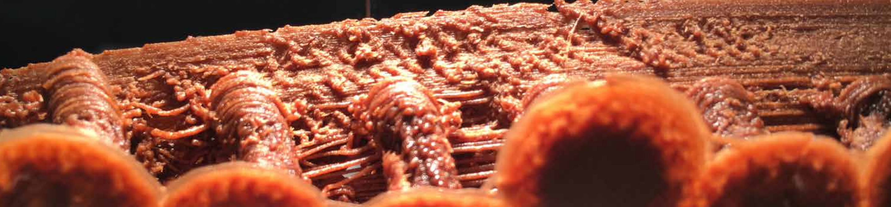
Image 3D Printed Cork Waste Substrate with engineered Fungi. Photo by Maria Paz Gutierrez
