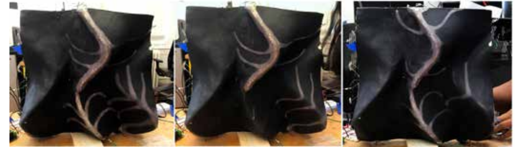
Image Sentient Concrete prototype showing variation of surface color change due to temperatures induced internally by electromechanical controls and external heat dissipation
