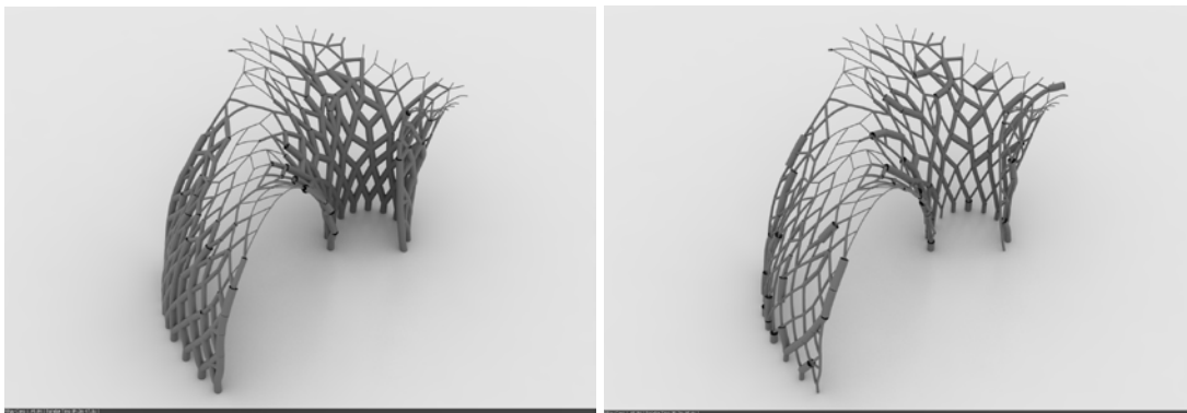
Figure 5 and 6: Layer Thicknesses (exaggerated) after initial specification and final ones after negotiation of required bending and FE analysis
