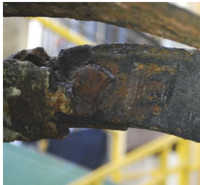
The hull interior was supported by half-moon shaped iron rings, joined with bolts and a slotted plate, tightened with wedges.
