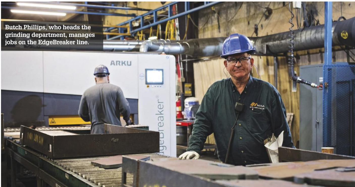
The EdgeBreaker 4000 is a two-sided deburring machine capable of dual-sided rounding and deburring.
