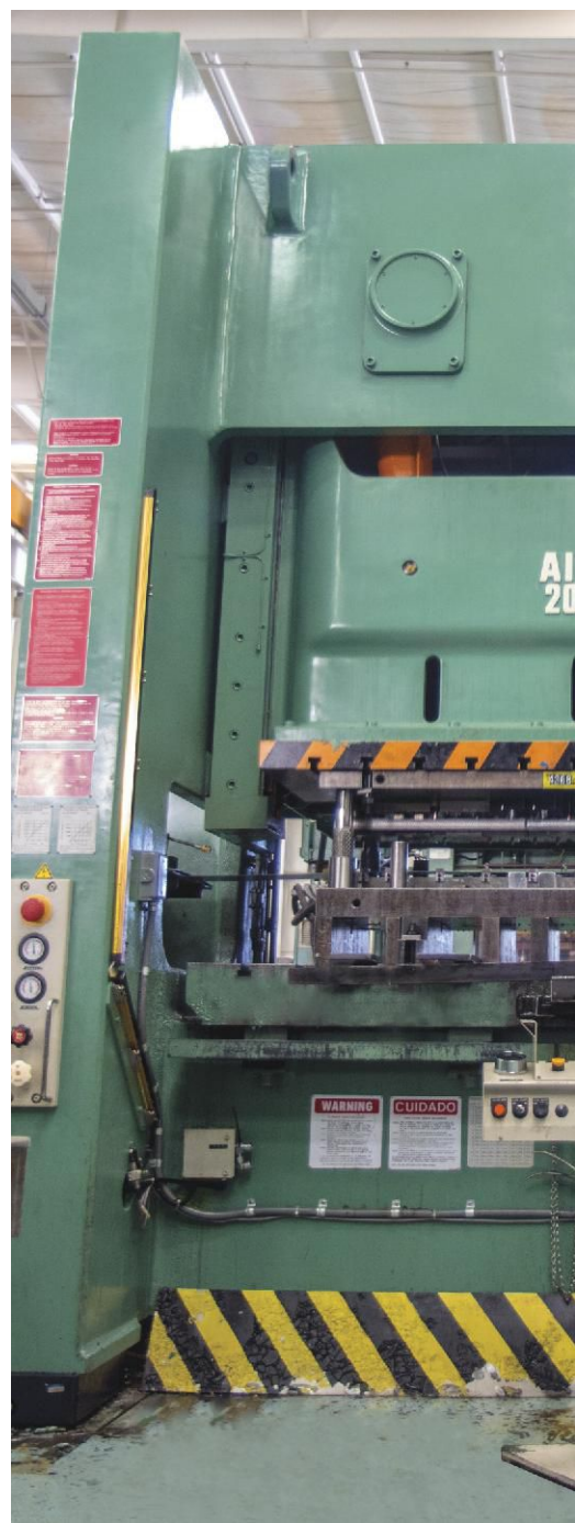
An operator uses step feed to test the die and watch the part form in real time.
