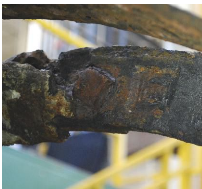
The hull interior was supported by half-moon shaped iron rings, joined with bolts and a slotted plate, tightened with wedges.
