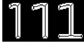
Figure 8: Symbol complexity. The complexity of each character is quantified by the length of each digit's morphological skeleton (example with a height of 41 pixels). The longer the string, the more complex the character.
