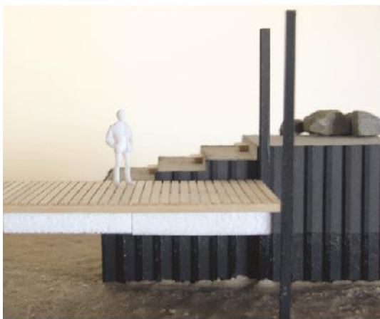
Image 16: As the tide rises, the floating dock eventually meets the steps at the end of the pier.
