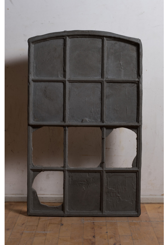
The window cast in concrete. Going from points to concrete requires several steps and translations. Eventually, the casting becomes a representation of the digital point cloud.
