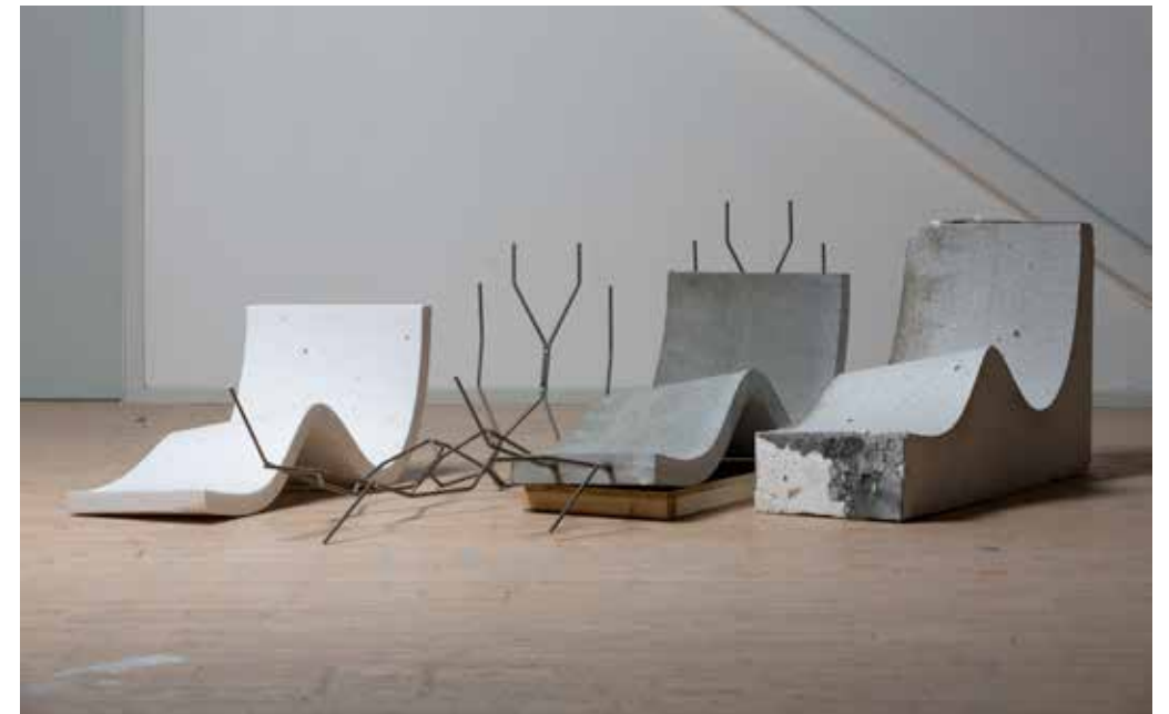
From left to right: Positive EPS shape left over from cutting, rebar element, concrete with rebar element inside, and used formwork. The lineup shows some of the involved processes and how they correspond.
