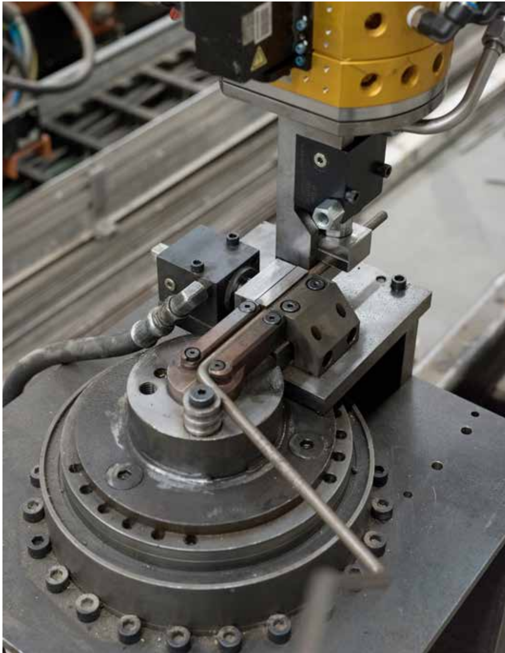
Close-up of the robot's end effector and the external axis with the bender die. The final bent angle is the combined result of the bending angle and the material springback. The bending setup is a custom installation made by FABLab Director Wes McGee et al.
