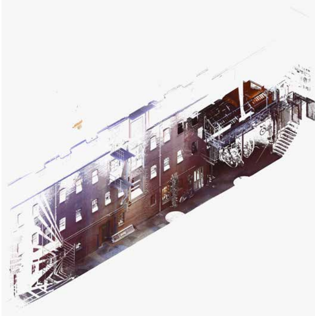
Axonometric section view through the point cloud representation of the scanned alley. The scanning is focused around a series of windows on the ground floor.
