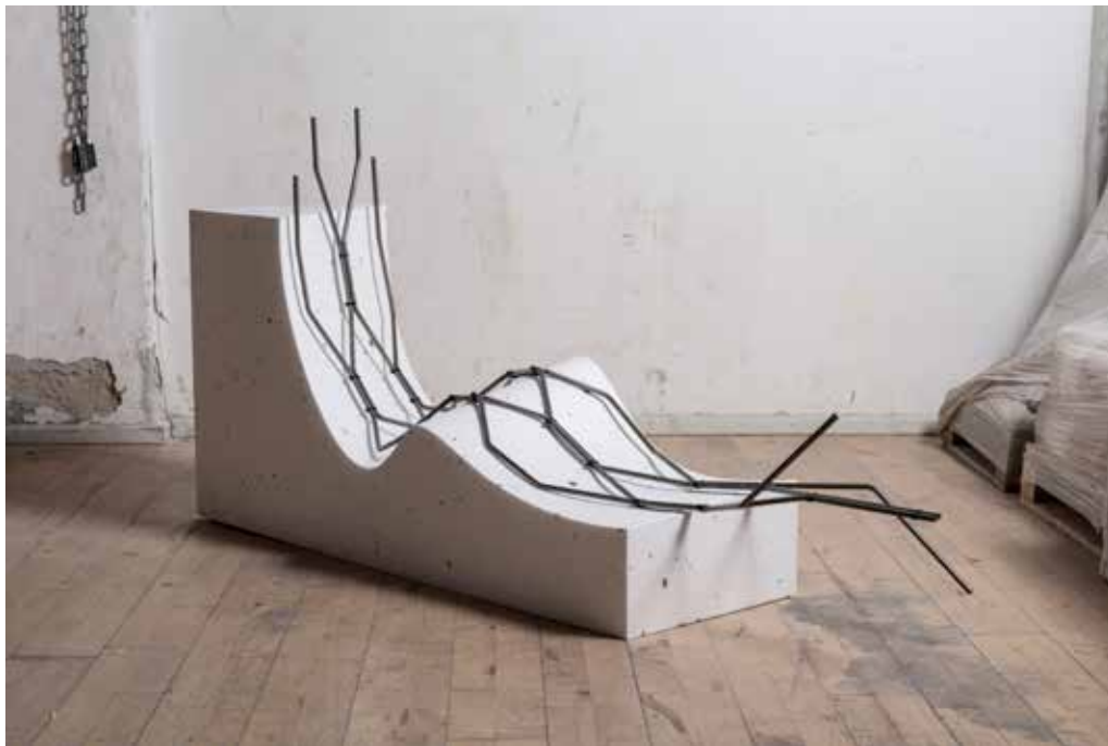
Assembled rebar steel and EPS formwork. Even though both a bending process and hot wire cutting tolerances can be improved, the formwork surface and steel structure closely follow each other.
