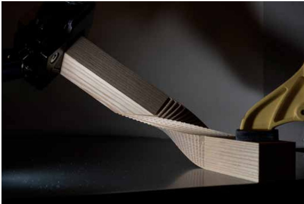
Complex kerf bending: Digital drawing and fabrication combined bring another perspective to the term wood bending.
