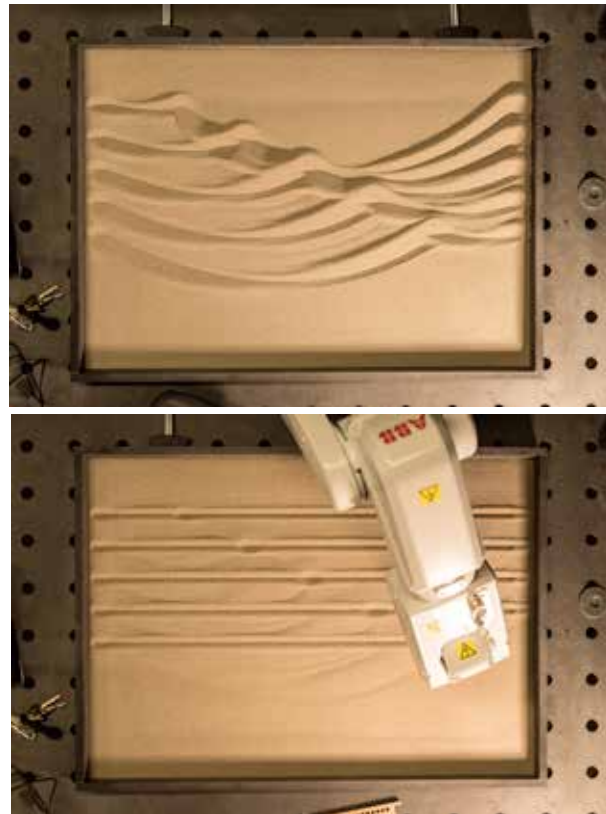
Joint interpolated motion and straight-line interpolated motion compared. Top figure illustrates the drawing information from which the code is extracted. Five sets of two curves describe the processing. Each of the five sets holds three points - those points define the code. The robot moves the end-effector from point to point using different interpolation strategies. The middle photo shows how the robot connects the points using joint interpolation ( MoveJ ). The lower photo shows the robot using straight-line interpolation ( MoveL ). In this case, the straight-line interpolation closely resembles the source geometry, whereas the joint interpolated motion adds an entirely new interpretation of the connected points.
