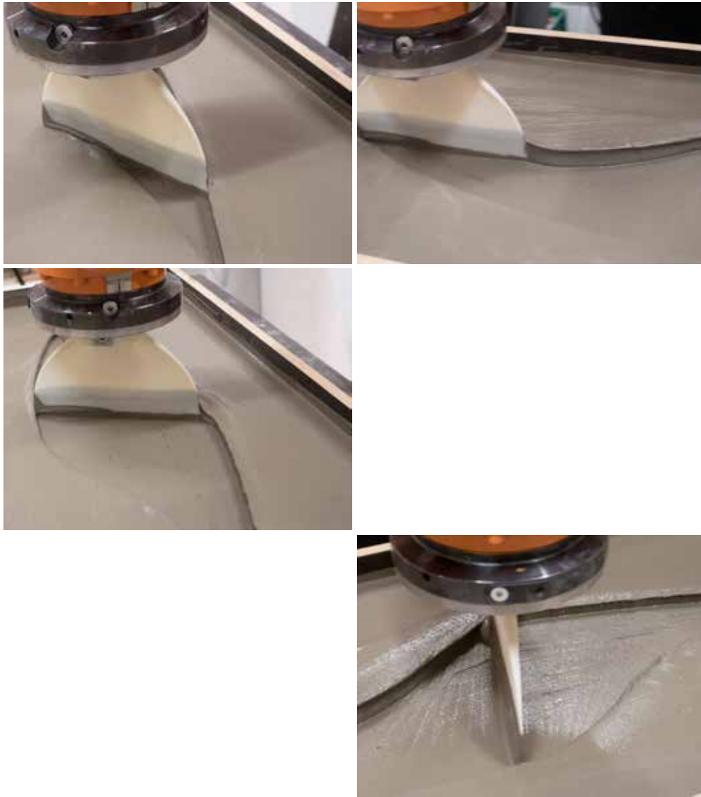
End-effectors working in the concrete. Size, shape, and configuration of the end-effector will impact the reactions and appearance of the concrete.
