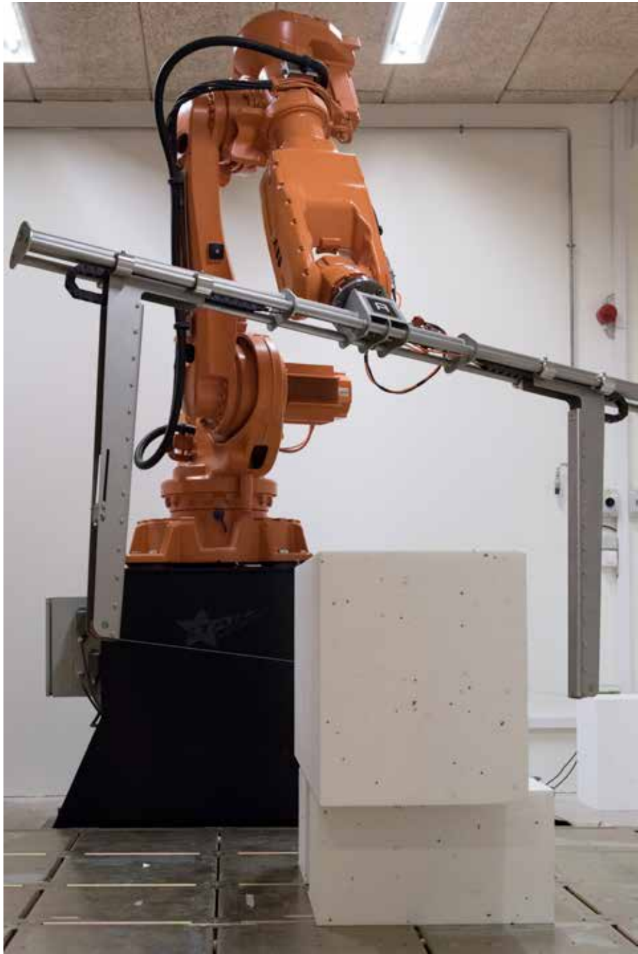
Hot wire cutting at the robot lab at Aarhus School of Architecture
