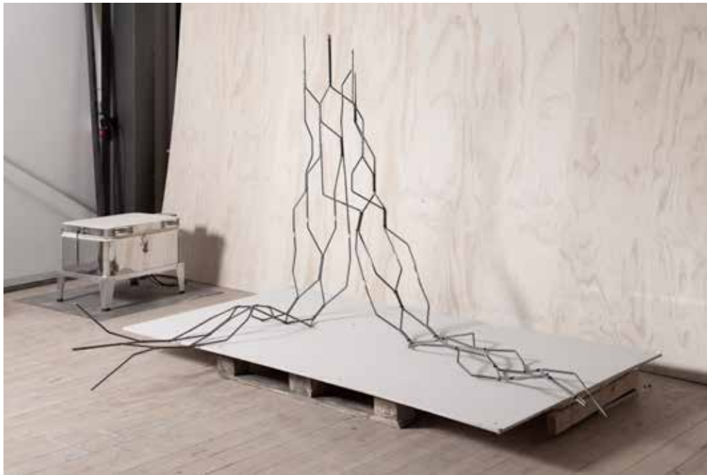
Combined concrete and steel hybrid construction - before concrete casting. Two reinforced, curved concrete slabs morph into a steel truss beam.
