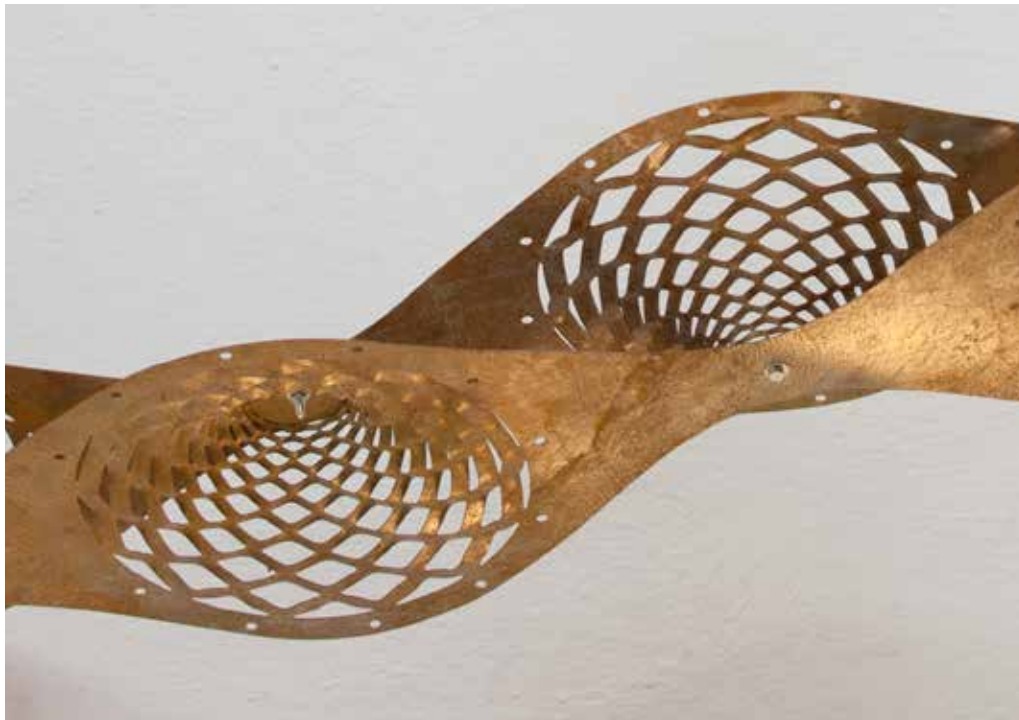
A composition of stretched steel objects supporting each other. The result is a fixed beam-like fragment with little weight and high strength. A varying approach to material machining and material capacities is not limited to each element, but extends into the combination and composition of those elements into possible, larger components or structures.
