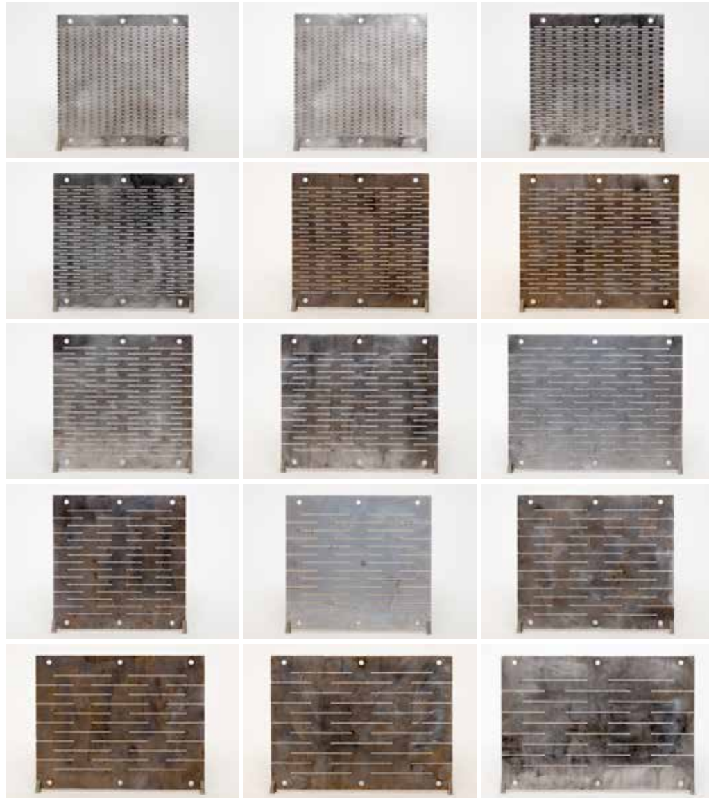
Systematic testing of different sizes of slits. Finding the material limits was necessary for building the process.
