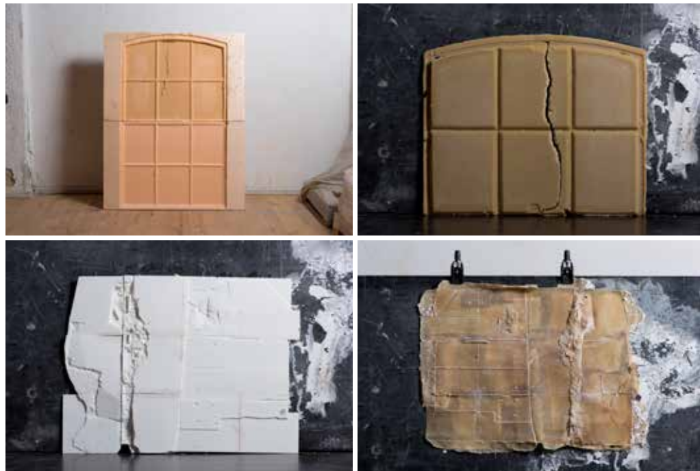
Different fabrications made from scanings of the alley: CNC-milled foam, beeswax casting, SLS 3D print of texture collage and latex casting of the collage.
