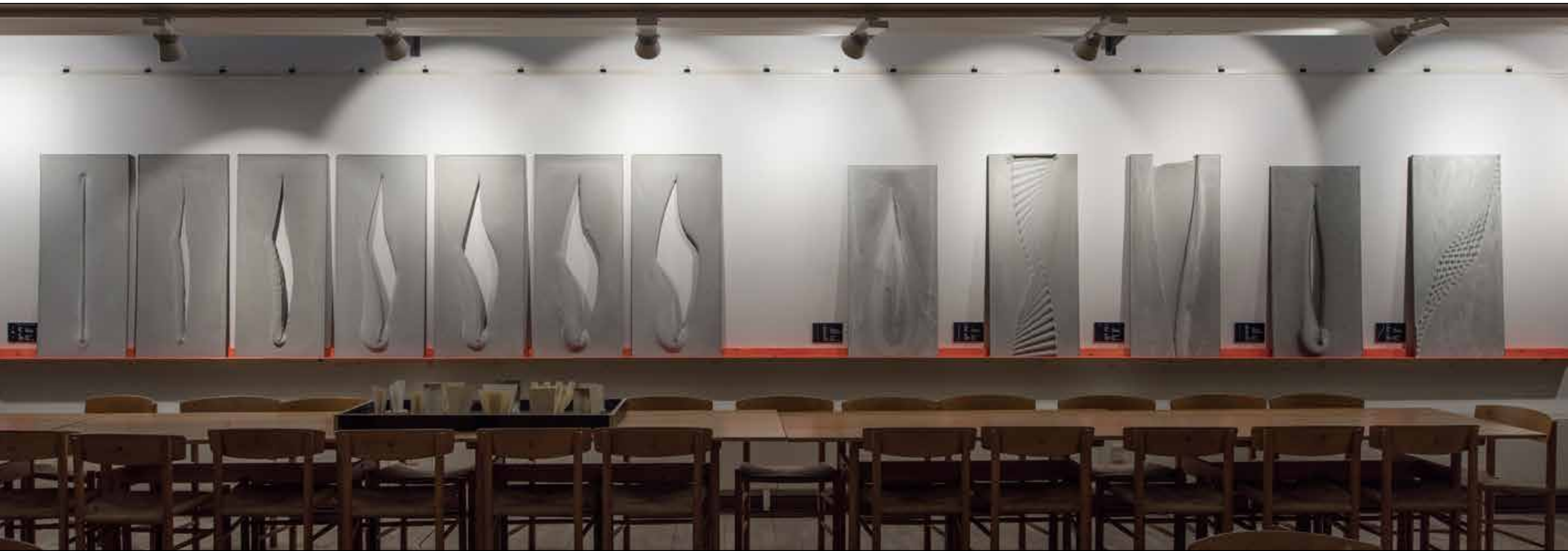
Concrete panels exhibited in the canteen at Aarhus School of Architecture. Left side shows a serial investigation where a gradually increasing rotation of a mid-plane opens up the concrete panel by panel. The right side shows individual, scattered explorations either focusing on robotic movement or variables in the concrete mixing and handling. On an opposite wall, the short movie was showing selected close-ups from the process.
