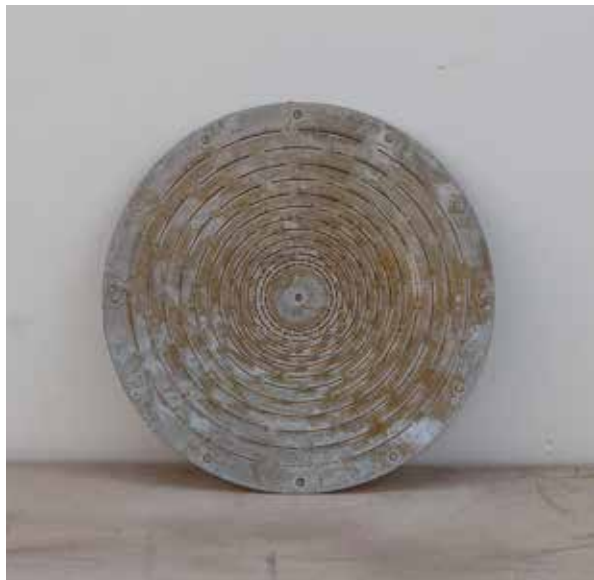
Cutting path geometry, cut steel, stretching, three-dimensional result.
