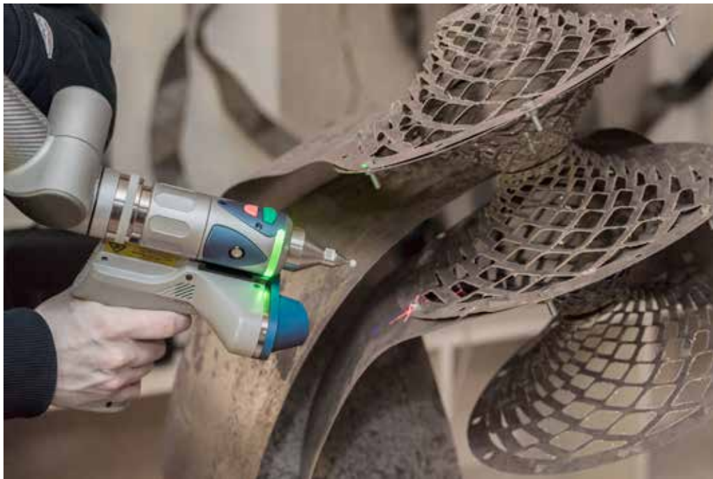
Different techniques can be used for 3D scanning or digitisation of physical objects. In this experiment, two types of laser scanners were used. A Faro Focus for spatial registration and a, as shown in the photo, Faro Edge handheld scanner for objects and details. The process allows digital extraction of geometries and curvatures created in physical space.
