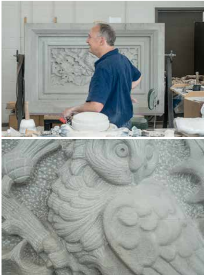
Photos taken during visit at CIMS. Here stonemason Phil White is finishing the robotic milled sandstone relief. Close up shows the difference between manual finish and robotic roughening.
