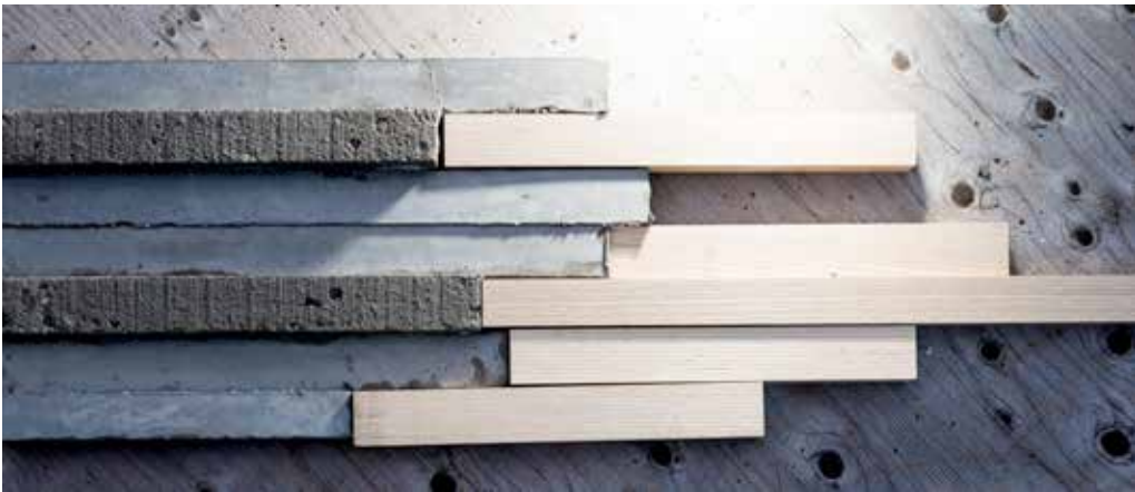
The long grains of the ash wood are sought to be combined with the solidified homogeneity of the concrete. Different surface treatments for the concrete are tested out.
