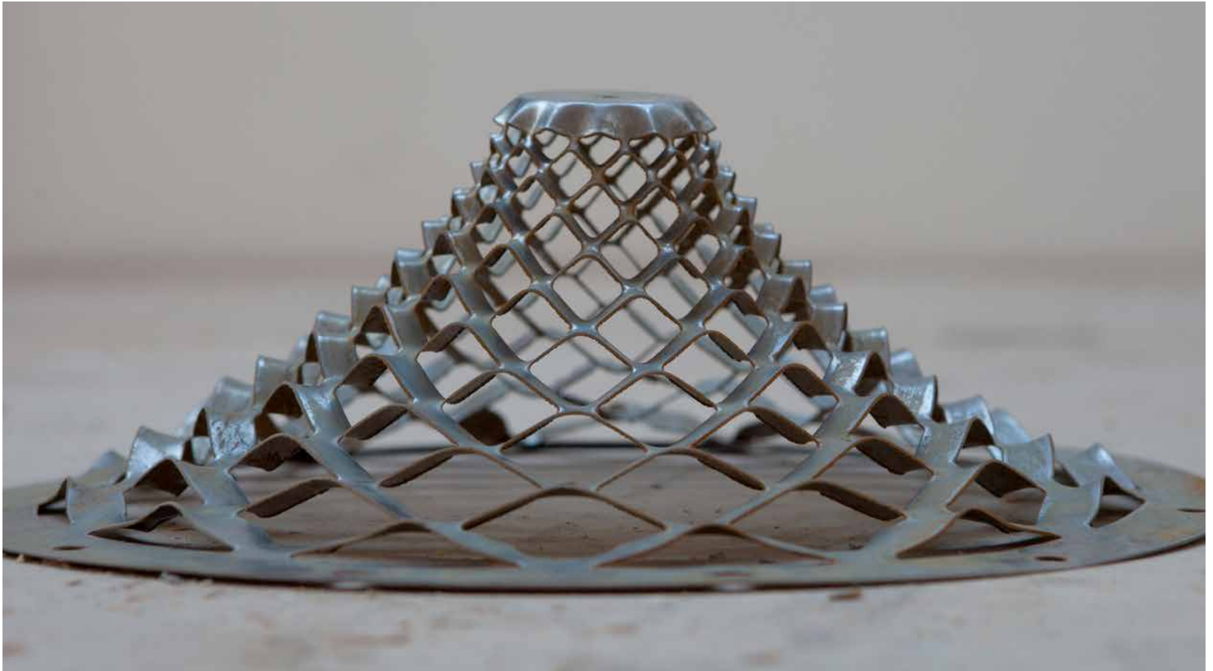
The overall geometry and multitude of small plastic deformations create an unyielding three-dimensional, spatial object deriving from a flat piece of steel and two-dimensional machining data.
