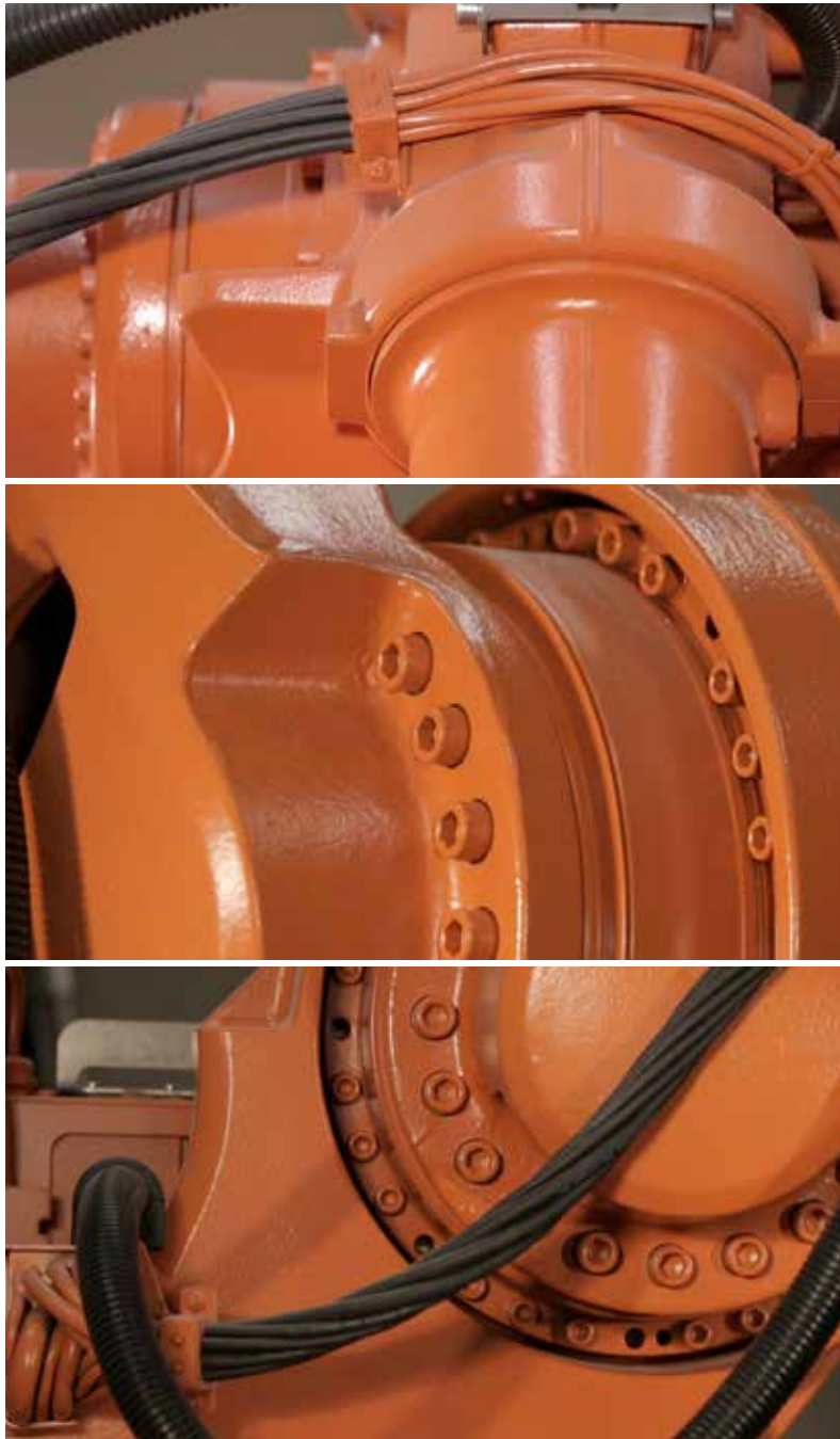
A total of 6 mechanical axes defines the freedom of motion for the robotic arm. The interplay among the axes composes the movement of the end-effector.
