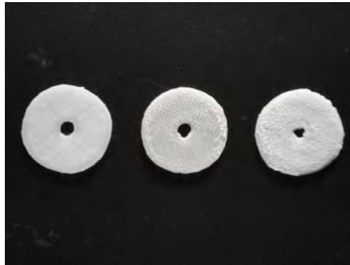
Figure 6. Prototype pieces printed from control widget 1 using recyclable PLA filament. Best to poorest quality resolution reading from left to right.
