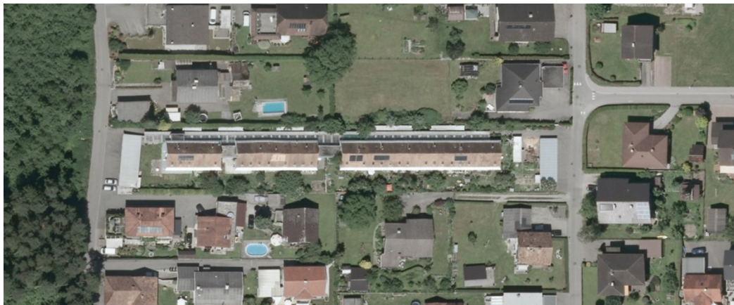
Fig. 1 The long site is situated close to a beautiful forest in an area, where only space consuming one-family homes existed. There are carports at the eastern and the western end of the site with no car access to the units. The project is structured in 6+3+2 units, connected by a 105 meters long corridor in the north. The gaps are partly filled with a community house and an office.
