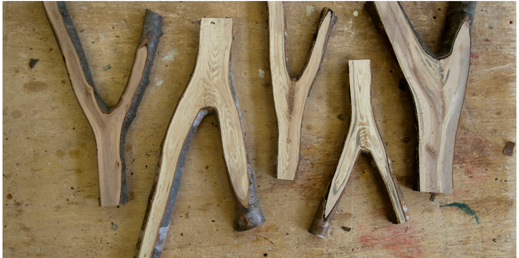
Figure 6 Individual branches only captured by the distance between two planed parallel surfaces (M Bereuter).
