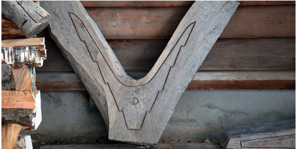
Figure 3 The form of a jig for a Viking longship rib applied to a naturally grown fork (Viking Ship Museum Roskilde).
